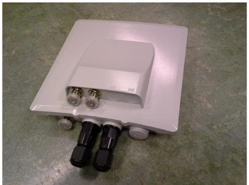
Picture 7: EUT type InfiLINK XG Um. External antenna 28 dBi, 4.9-6.425 GHz Band
