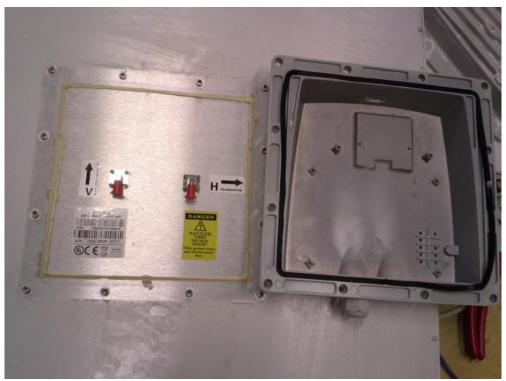
Picture 31: EUT R5000-Smn. Antenna 28 dBi, 4.9-6.425 GHz Band. No trace of water or dust inside the enclosure after the IP6X, IPX6 and IPX7 tests.
