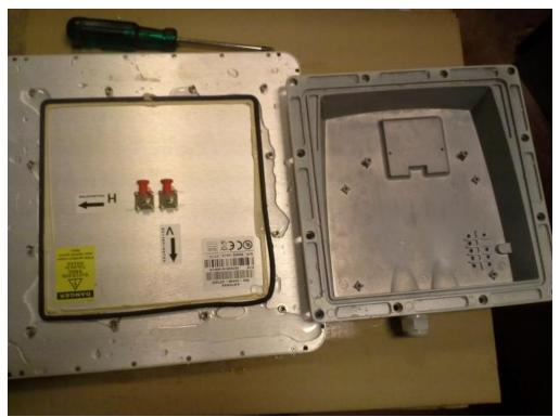
Picture 30: EUT R5000-Smn. Antenna 21 dBi, 4.9-6.425 GHz Band. No trace of water or dust inside the enclosure after the IP6X, IPX6 and IPX7 tests.
