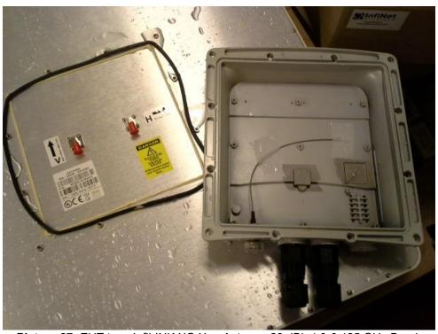
**Picture 27:** EUT type InfiLINK XG Xm. Antenna 28 dBi, 4.9-6.425 GHz Band. No trace of water or dust inside the enclosure after the IP6X, IPX6 and IPX7 tests.
