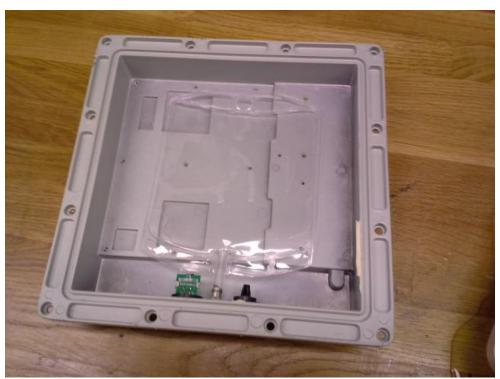
Picture 25: EUT type R5000-Mmx. Antenna 23 dBi, 3.4-6.425 GHz Band. No trace of water inside the enclosure after the IPX7 test.
