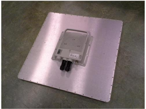
Picture 6: EUT type InfiLINK XG Xm. Antenna 28 dBi, 4.9-6.425 GHz Band
