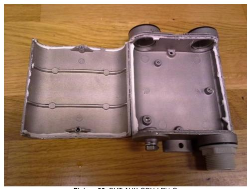
Picture 33: EUT AUX-ODU-LPU-G No trace of water or dust inside the enclosure after the IP6X, IPX6 and IPX7 tests.
