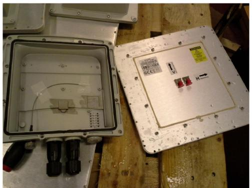
Picture 26: EUT type InfiLINK XG Xm. Antenna 23 dBi, 4.9-6.425 GHz Band. No trace of water or dust inside the enclosure after the IP6X, IPX6 and IPX7 tests.
