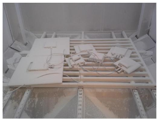
Picture 20: EUTs after IP6X test (Dust with underpressure)
