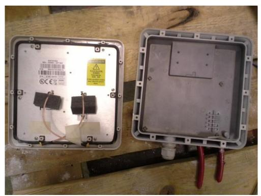
Picture 29: EUT R5000-Smn. Antenna 19 dBi, 4.9-6.425 GHz Band. No trace of water or dust inside the enclosure after the IP6X, IPX6 and IPX7 tests.
