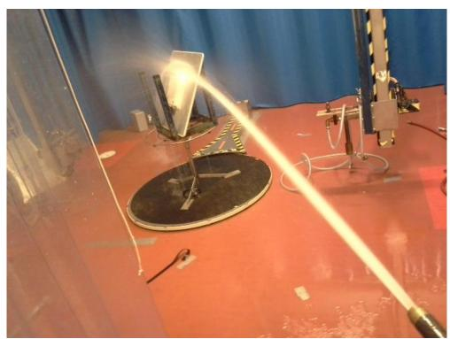
Picture 23: Example of EUT during IPX6 test
