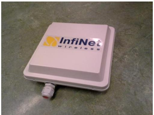
Picture 9: EUT R5000-Smn. Antenna 19 dBi, 4.9-6.425 GHz Band
