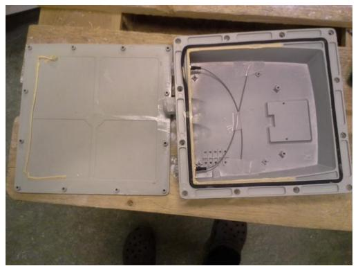
Picture 32: EUT R5000-Lmn. External antenna, 3.4-6.425 GHz Band. No trace of water or dust inside the enclosure after the IP6X, IPX6 and IPX7 tests.
