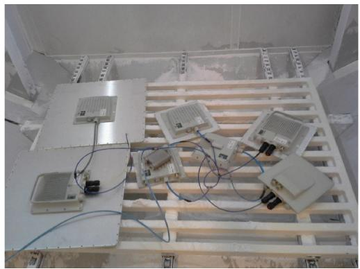
Picture 19: EUTs before IP6X test (Dust with underpressure)
