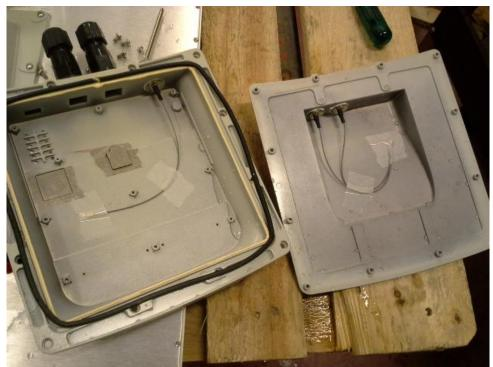
Picture 28: EUT type InfiLINK UG Xm. External antenna. 4.9-6.425 GHz Band. No trace of water or dust inside the enclosure after the IP6X, IPX6 and IPX7 tests.
