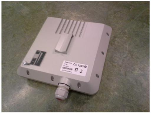
Picture 10: EUT R5000-Smn. Antenna 19 dBi, 4.9-6.425 GHz Band
