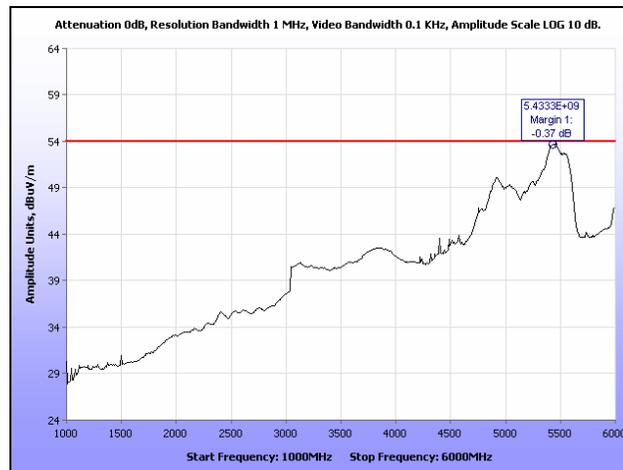
Plot 212. Radiated Spurious Emissions, High Channel, 40 MHz, 1 GHz – 6 GHz, Average, 23 dBi
