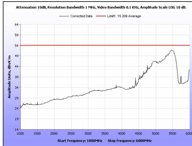
Plot 120. Radiated Spurious Emissions, Low Channel, 20 MHz, 1 GHz – 6 GHz, Average, 19 dBi
