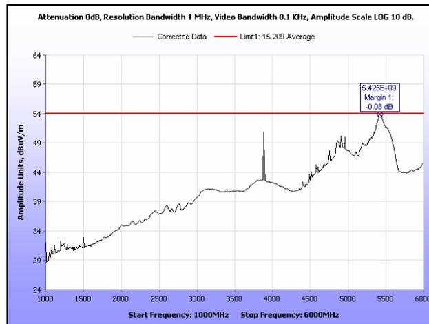
**Plot 200. Radiated Spurious Emissions, High Channel, 40 MHz, 1 GHz – 6 GHz, Average, 21 dBi**
