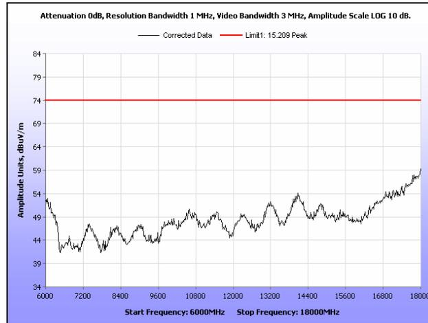
Plot 123. Radiated Spurious Emissions, Low Channel, 20 MHz, 6 GHz – 18 GHz, Peak, 19 dB
