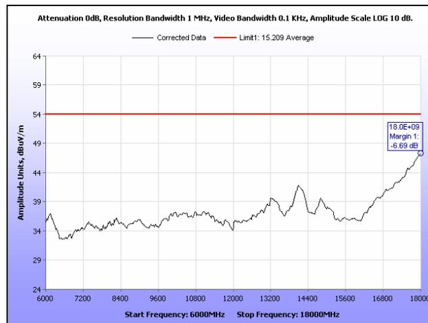
Plot 218. Radiated Spurious Emissions, Low Channel, 40 MHz, 6 GHz – 18 GHz, Peak, 28 dBi
