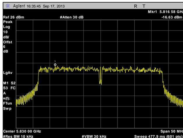
**Plot 325. Peak Power Spectral Density, High Channel, Point to Multi-Point, 40 MHz, Port 2, 21 dBi**
