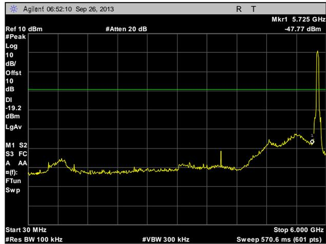
Plot 262. Conducted Spurious Emissions, High Channel, 40 MHz, Port 2, 30 MHz – 6 GHz
