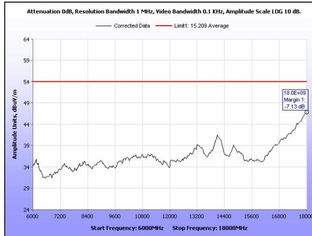
Plot 222. Radiated Spurious Emissions, Mid Channel, 40 MHz, 6 GHz – 18 GHz, Peak, 28 dBi
