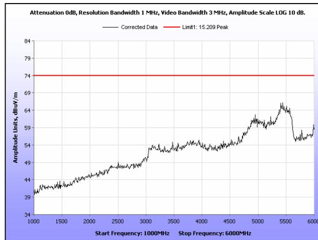
Plot 149. Radiated Spurious Emissions, Mid Channel, 20 MHz, 1 GHz – 6 GHz, Peak, 23 dB
