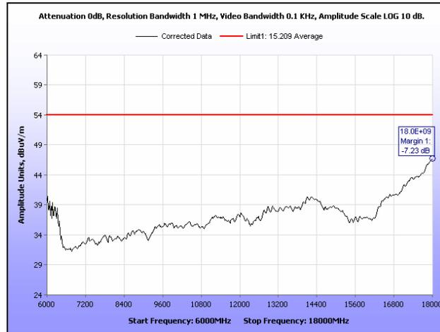
Plot 114. Radiated Spurious Emissions, Mid Channel, 20 MHz, 6 GHz – 18 GHz, Average, 16 dBi
