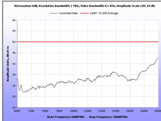
**Plot 198. Radiated Spurious Emissions, Mid Channel, 40 MHz, 6 GHz – 18 GHz, Average, 21 dBi**
