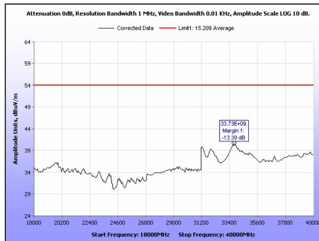
**Plot 230. Radiated Spurious Emissions, Mid Channel, 20 MHz, 18 GHz – 40 GHz, Average**
