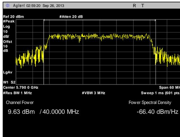
**Plot 76. Peak Power Output, Point to Multi-Point, Mid Channel, 40 MHz, Port 1, Port 1, 19 dBi**
