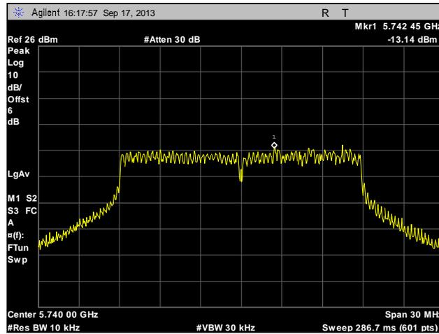
**Plot 287. Peak Power Spectral Density, Low Channel, Point to Multi-Point, 20 MHz, Port 2, 16 dBi**
