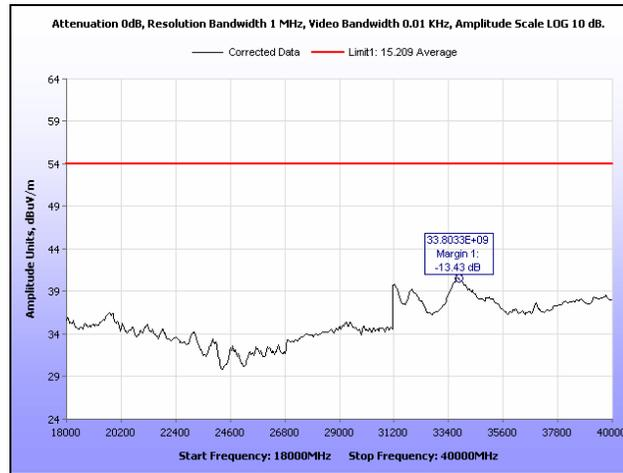
**Plot 234. Radiated Spurious Emissions, Low Channel, 40 MHz, 18 GHz – 40 GHz, Average**
