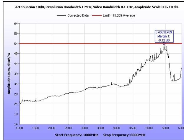
Plot 180. Radiated Spurious Emissions, Low Channel, 40 MHz, 1 GHz – 6 GHz, Average, 19 dBi
