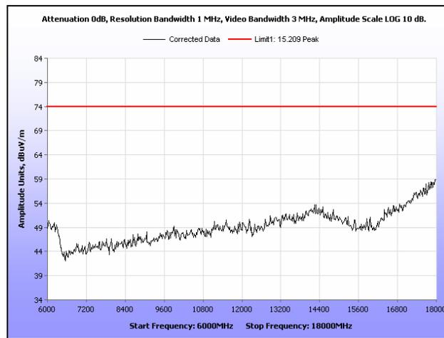
Plot 115. Radiated Spurious Emissions, Mid Channel, 20 MHz, 6 GHz – 18 GHz, Peak, 16 dBi
