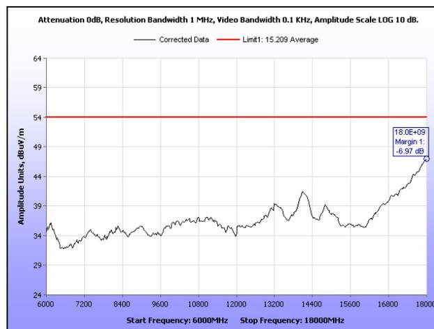
**Plot 158. Radiated Spurious Emissions, Low Channel, 20 MHz, 6 GHz – 18 GHz, Average, 28 dBi**
