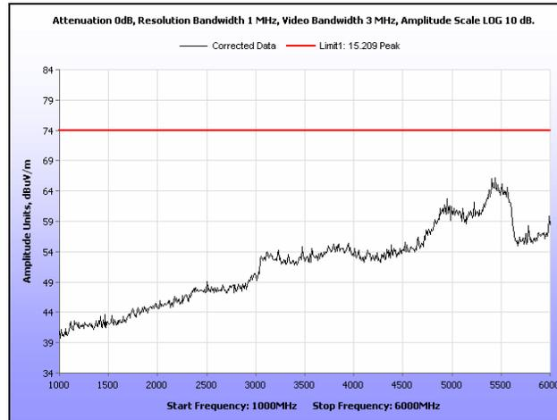
**Plot 153. Radiated Spurious Emissions, High Channel, 20 MHz, 1 GHz – 6 GHz, Peak, 23 dBi**
