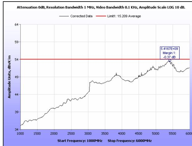
Plot 216. Radiated Spurious Emissions, Low Channel, 40 MHz, 1 GHz – 6 GHz, Average, 28 dBi
