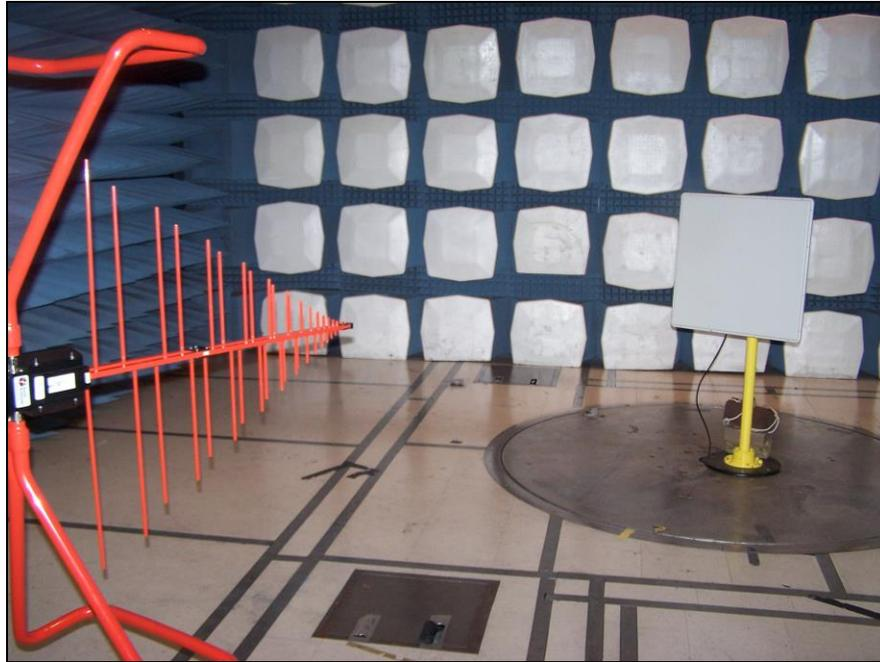
**Photograph 5. Radiated Spurious Emissions, Test Setup, 30 MHz – 1 GHz**
