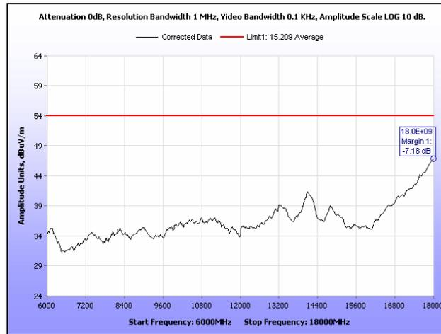
**Plot 166. Radiated Spurious Emissions, High Channel, 20 MHz, 6 GHz – 18 GHz, Average, 28 dB**
