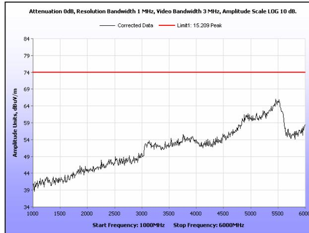
**Plot 189. Radiated Spurious Emissions, High Channel, 40 MHz, 1 GHz – 6 GHz, Peak, 19 dBi**
