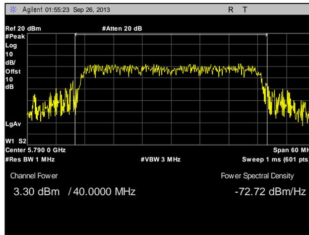
**Plot 100. Peak Power Output, Point to Multi-Point, Mid Channel, 40 MHz, Port 2, 28 dBi**
