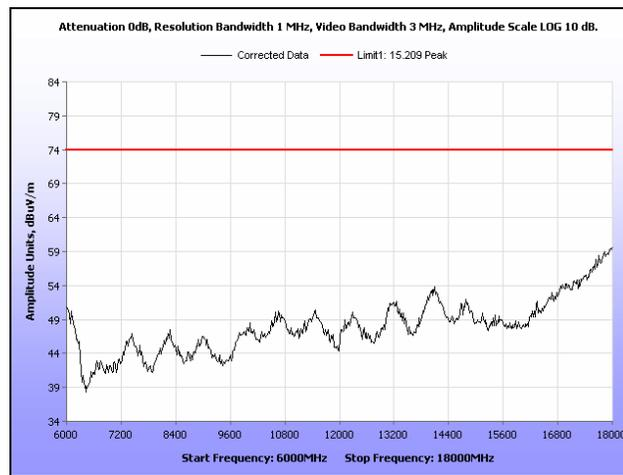
**Plot 151. Radiated Spurious Emissions, Mid Channel, 20 MHz, 6 GHz – 18 GHz, Peak, 23 dBi**
