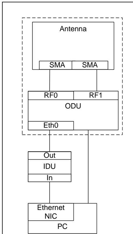
**Figure 1. Block Diagram of Test Configuration**
