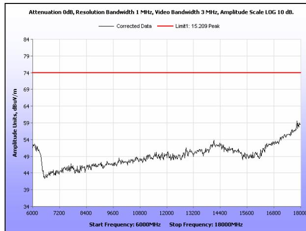
**Plot 179. Radiated Spurious Emissions, High Channel, 40 MHz, 6 GHz – 18 GHz, Peak, 16 dBi**
