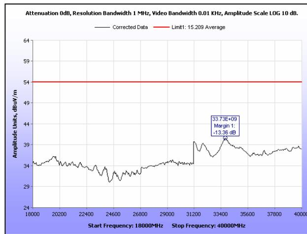
**Plot 232. Radiated Spurious Emissions, High Channel, 20 MHz, 18 GHz – 40 GHz, Average**
