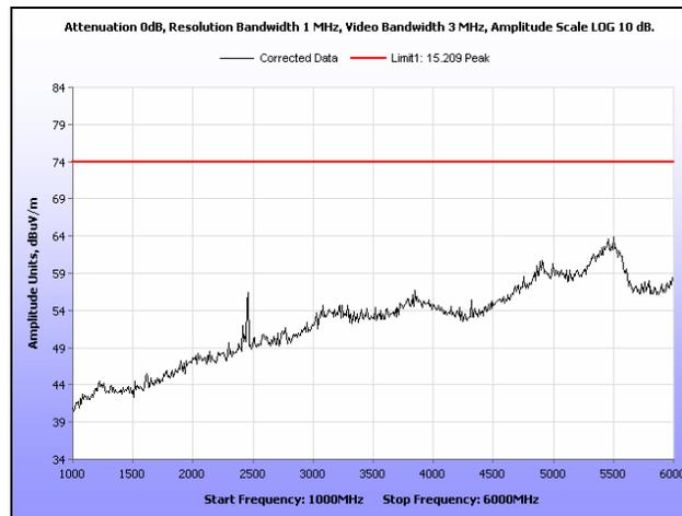
Plot 113. Radiated Spurious Emissions, Mid Channel, 20 MHz, 1 GHz – 6 GHz, Peak, 16 dB
