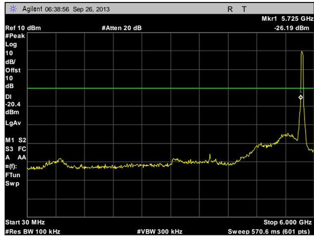
**Plot 252. Conducted Spurious Emissions, Low Channel, 40 MHz, Port 1, 30 MHz – 6 GHz**
