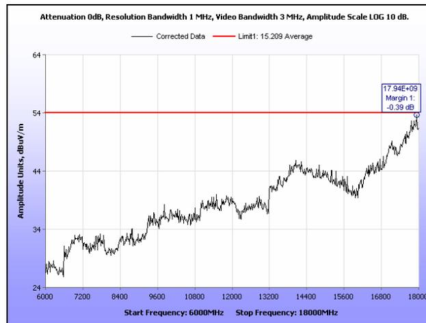
**Plot 191. Radiated Spurious Emissions, High Channel, 40 MHz, 6 GHz – 18 GHz, Peak, 19 dBi**
