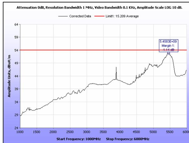
Plot 176. Radiated Spurious Emissions, High Channel, 40 MHz, 1 GHz – 6 GHz, Average, 16 dBi
