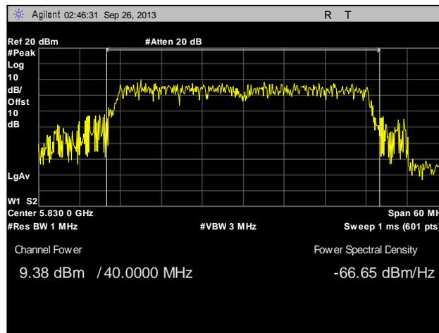
**Plot 98. Peak Power Output, Point to Multi-Point, High Channel, 40 MHz, Port 2, 23 dBi**
