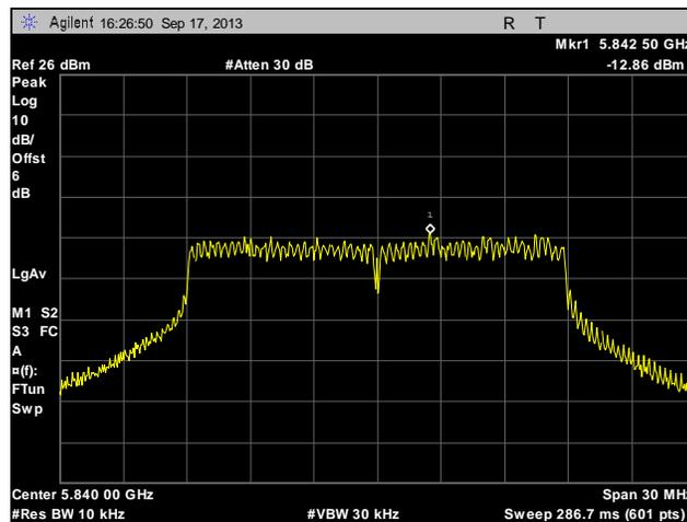
**Plot 295. Peak Power Spectral Density, High Channel, Point to Multi-Point, 20 MHz, Port 2, 21 dBi**
