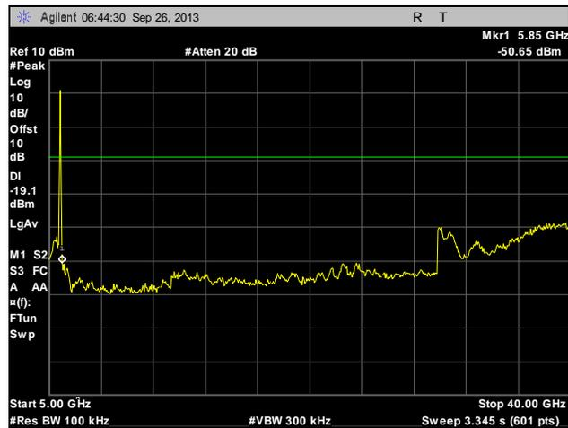
**Plot 259. Conducted Spurious Emissions, Low Channel, 40 MHz, Port 2, 5 GHz – 40 GHz**
