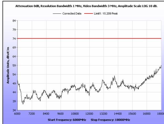
Plot 147. Radiated Spurious Emissions, Low Channel, 20 MHz, 6 GHz – 18 GHz, Peak, 23 dB
