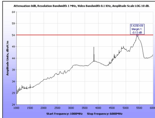
**Plot 192. Radiated Spurious Emissions, Low Channel, 40 MHz, 1 GHz – 6 GHz, Average, 21 dBi**
