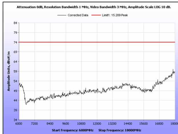
**Plot 119. Radiated Spurious Emissions, High Channel, 20 MHz, 6 GHz – 18 GHz, Peak, 16 dBi**
