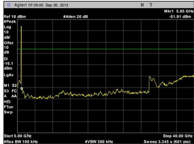
Plot 249. Conducted Spurious Emissions, Mid Channel, 20 MHz, Port 2, 5 GHz – 40 GHz
