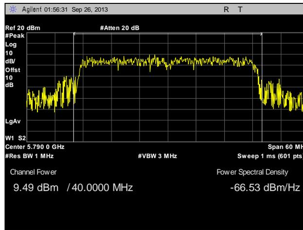
**Plot 94. Peak Power Output, Point to Multi-Point, Mid Channel, 40 MHz, Port 2, 21 dBi**
