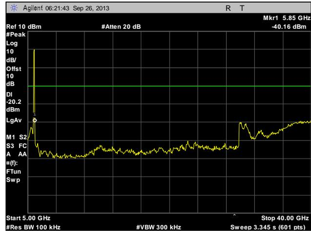
Plot 243. Conducted Spurious Emissions, Mid Channel, 20 MHz, Port 1, 5 GHz – 40 GHz
