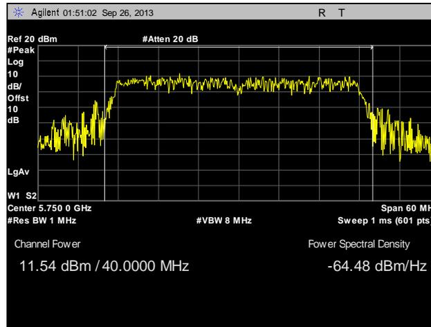
**Plot 87. Peak Power Output, Point to Multi-Point, Low Channel, 40 MHz, Port 2, 16 dBi**
