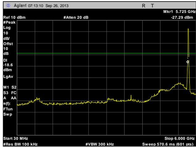
**Plot 246. Conducted Spurious Emissions, Low Channel, 20 MHz, Port 2, 30 MHz – 6 GHz**
