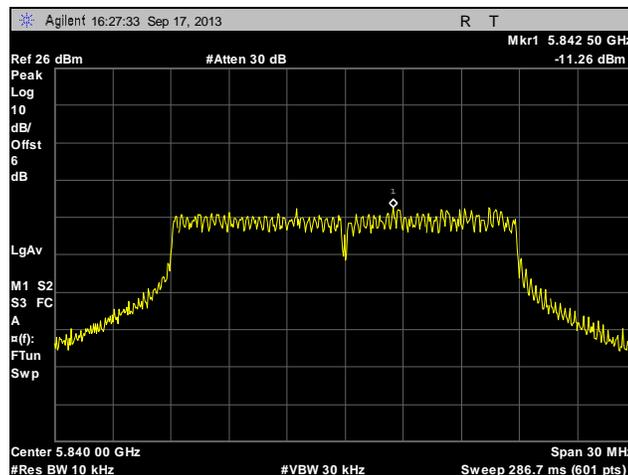
**Plot 289. Peak Power Spectral Density, High Channel, Point to Multi-Point, 20 MHz, Port 2, 16 dBi**
