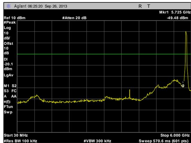
Plot 244. Conducted Spurious Emissions, High Channel, 20 MHz, Port 1, 30 MHz – 6 GHz
