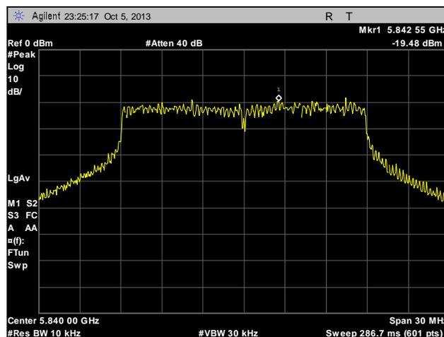
**Plot 301. Peak Power Spectral Density, High Channel, Point to Multi-Point, 20 MHz, Port 2, 28 dBi**
