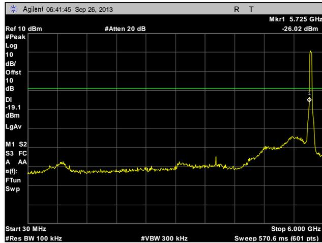
**Plot 258. Conducted Spurious Emissions, Low Channel, 40 MHz, Port 2, 30 MHz – 6 GHz**
