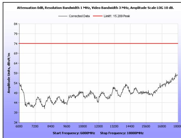
Plot 187. Radiated Spurious Emissions, Mid Channel, 40 MHz, 6 GHz – 18 GHz, Peak, 19 dBi
