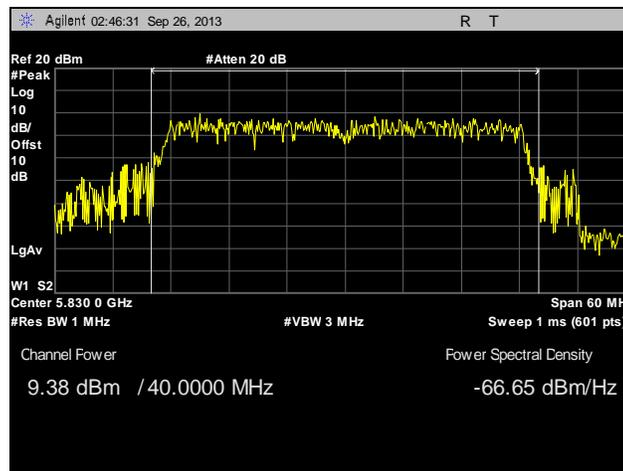
**Plot 92. Peak Power Output, Point to Multi-Point, High Channel, 40 MHz, Port 2, Port 2, 19 dBi**
