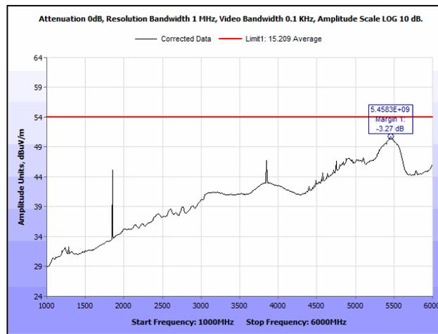
Plot 112. Radiated Spurious Emissions, Mid Channel, 20 MHz, 1 GHz – 6 GHz, Average, 16 dB
