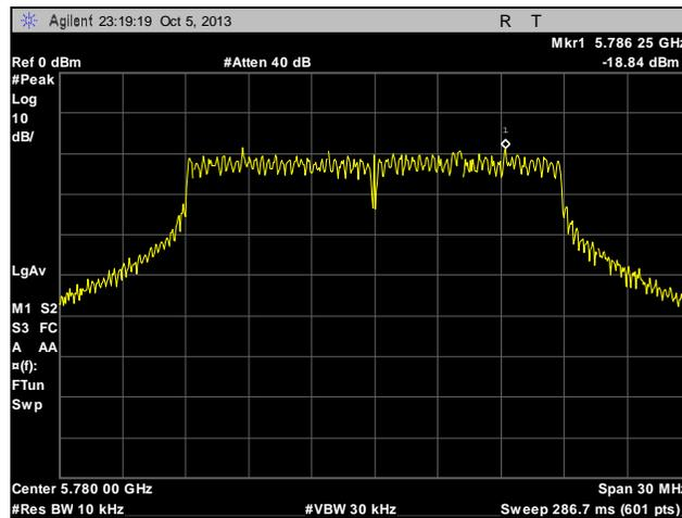
**Plot 285. Peak Power Spectral Density, Mid Channel, Point to Multi-Point, 20 MHz, Port 1, 28 dBi**
