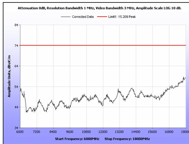
Plot 127. Radiated Spurious Emissions, Mid Channel, 20 MHz, 6 GHz – 18 GHz, Peak, 19 dBi
