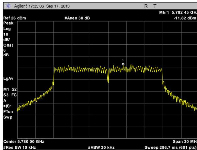
**Plot 276. Peak Power Spectral Density, Mid Channel, Point to Multi-Point, 20 MHz, Port 1, 19 dBi**
