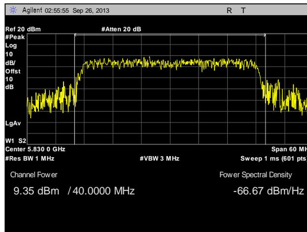
**Plot 77. Peak Power Output, Point to Multi-Point, High Channel, 40 MHz, Port 1, Port 1, 19 dBi**
