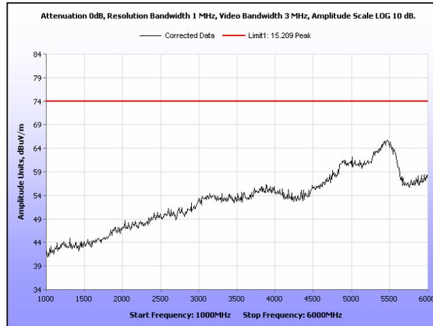
**Plot 177. Radiated Spurious Emissions, High Channel, 40 MHz, 1 GHz – 6 GHz, Peak, 16 dBi**
