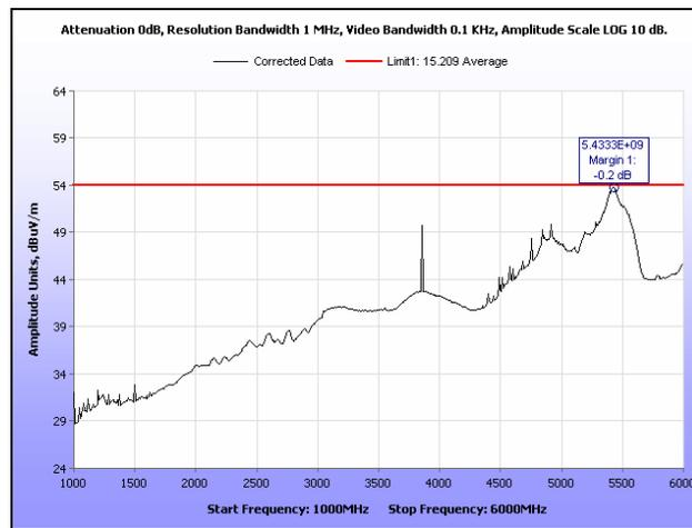
Plot 196. Radiated Spurious Emissions, Mid Channel, 40 MHz, 1 GHz – 6 GHz, Average, 21 dB
