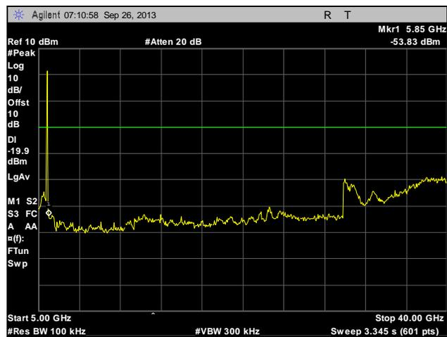
**Plot 247. Conducted Spurious Emissions, Low Channel, 20 MHz, Port 2, 5 GHz – 40 GHz**
