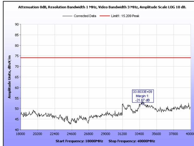
**Plot 231. Radiated Spurious Emissions, Mid Channel, 20 MHz, 18 GHz – 40 GHz, Peak**
