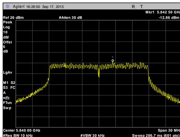
**Plot 292. Peak Power Spectral Density, High Channel, Point to Multi-Point, 20 MHz, Port 2, 19 dBi**
