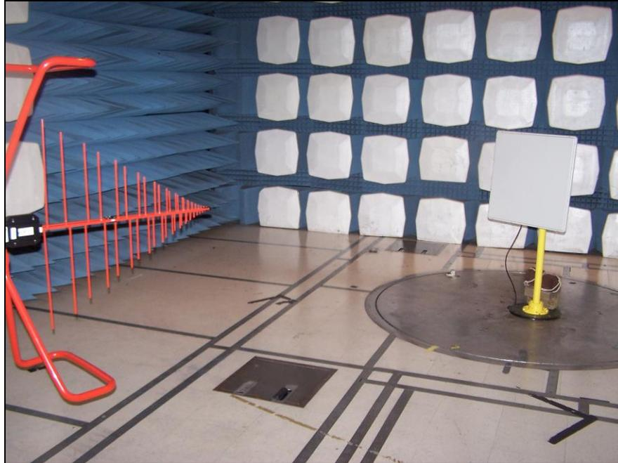
**Photograph 3. Radiated Emissions, Test Setup, 30 MHz – 1 GHz**
