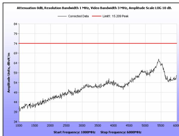
Plot 137. Radiated Spurious Emissions, Mid Channel, 20 MHz, 1 GHz – 6 GHz, Peak, 21 dB
