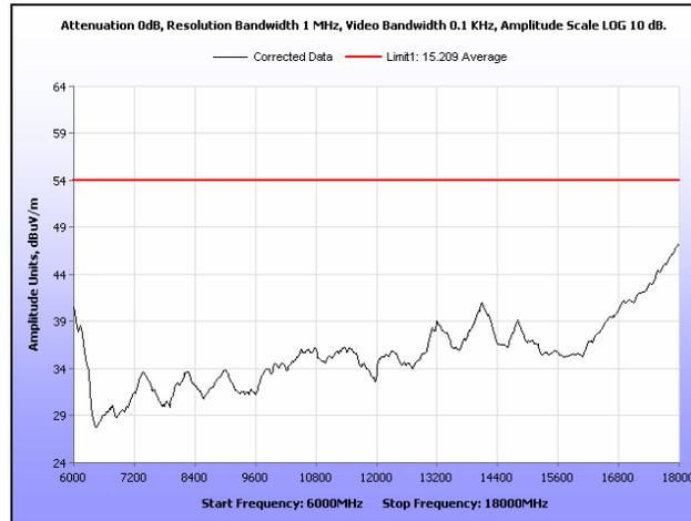
**Plot 150. Radiated Spurious Emissions, Mid Channel, 20 MHz, 6 GHz – 18 GHz, Average, 23 dBi**
