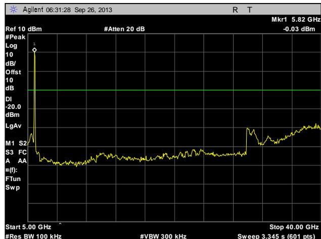
Plot 257. Conducted Spurious Emissions, High Channel, 40 MHz, Port 1, 5 GHz – 40 GHz
