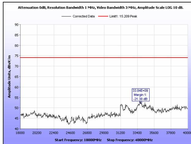
**Plot 239. Radiated Spurious Emissions, High Channel, 40 MHz, 18 GHz – 40 GHz, Peak**
