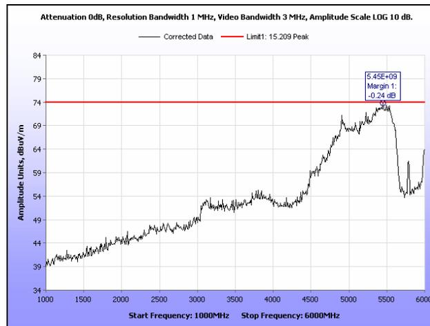
Plot 125. Radiated Spurious Emissions, Mid Channel, 20 MHz, 1 GHz – 6 GHz, Peak, 19 dB
