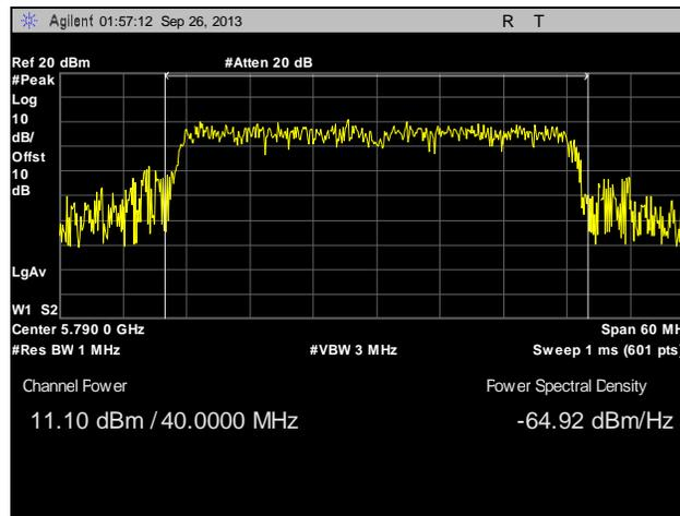
**Plot 88. Peak Power Output, Point to Multi-Point, Mid Channel, 40 MHz, Port 2, Port 2, 16 dBi**
