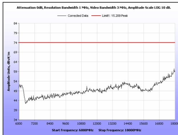
Plot 175. Radiated Spurious Emissions, Mid Channel, 40 MHz, 6 GHz – 18 GHz, Peak, 16 dBi
