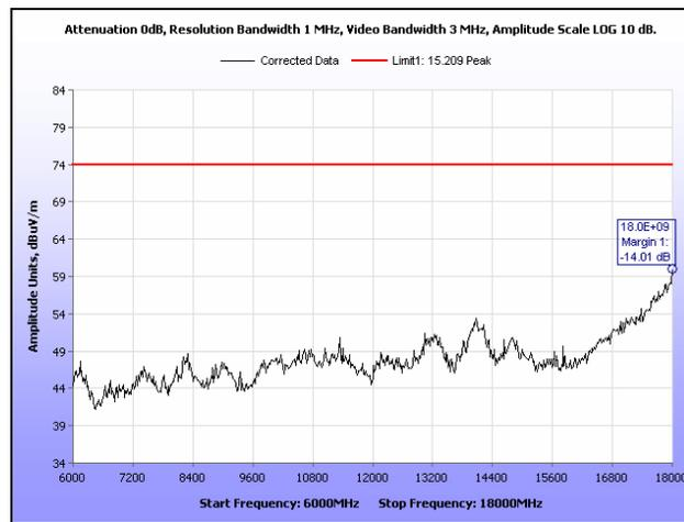
**Plot 163. Radiated Spurious Emissions, Mid Channel, 20 MHz, 6 GHz – 18 GHz, Peak, 28 dBi**
