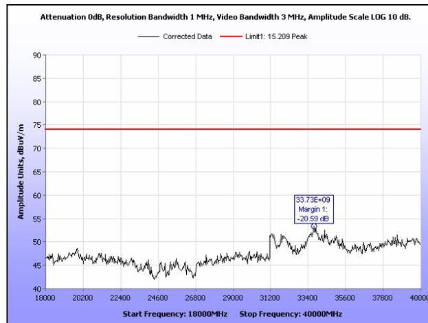
**Plot 233. Radiated Spurious Emissions, High Channel, 20 MHz, 18 GHz – 40 GHz, Peak**
