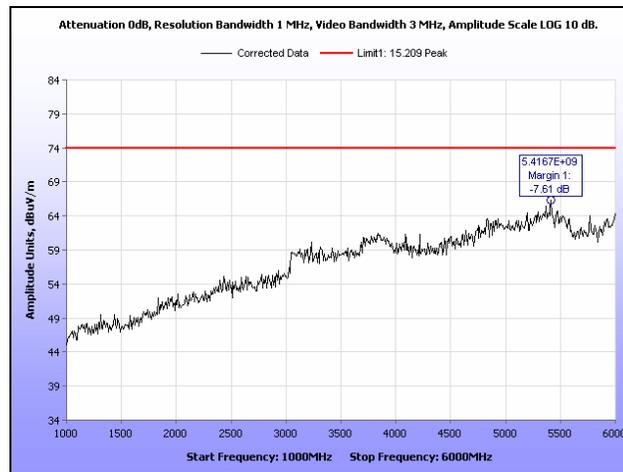
Plot 221. Radiated Spurious Emissions, Mid Channel, 40 MHz, 1 GHz – 6 GHz, Peak, 28 dB
