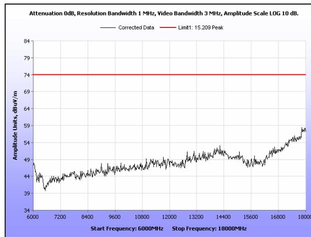
**Plot 139. Radiated Spurious Emissions, Mid Channel, 20 MHz, 6 GHz – 18 GHz, Peak, 21 dBi**
