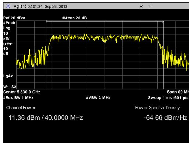
**Plot 89. Peak Power Output, Point to Multi-Point, High Channel, 40 MHz, Port 2, Port 2, 16 dBi**
