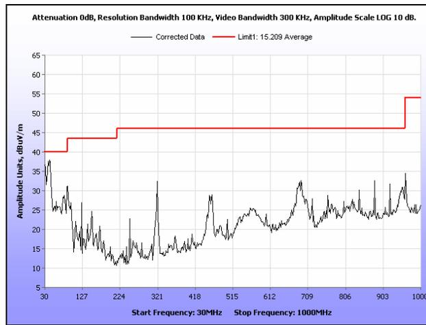
**Plot 103. Radiated Spurious Emissions, Mid Channel, 20 MHz, 30 MHz – 1 GHz, Peak**
