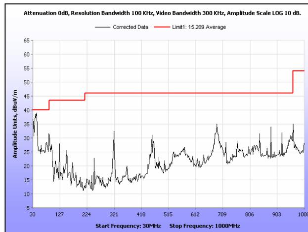
Plot 107. Radiated Spurious Emissions, High Channel, 40 MHz, 30 MHz – 1 GHz, Peak
