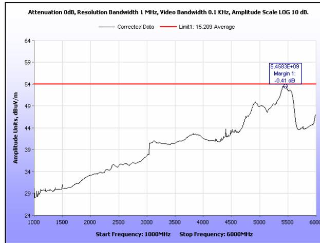
**Plot 204. Radiated Spurious Emissions, Low Channel, 40 MHz, 1 GHz – 6 GHz, Average, 23 dBi**
