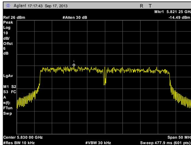
**Plot 307. Peak Power Spectral Density, High Channel, Point to Multi-Point, 40 MHz, Port 1, 19 dBi**
