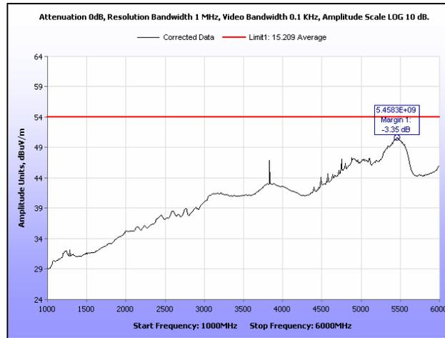
**Plot 168. Radiated Spurious Emissions, Low Channel, 40 MHz, 1 GHz – 6 GHz, Average, 16 dBi**
