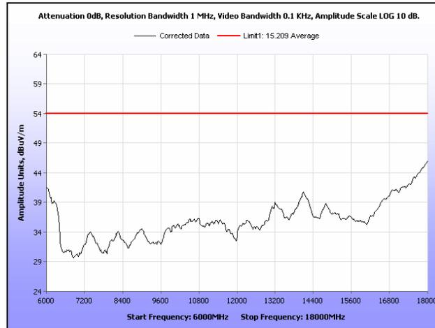
Plot 186. Radiated Spurious Emissions, Mid Channel, 40 MHz, 6 GHz – 18 GHz, Average, 19 dBi
