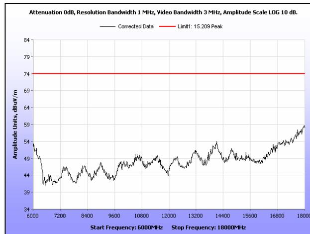
**Plot 131. Radiated Spurious Emissions, High Channel, 20 MHz, 6 GHz – 18 GHz, Peak, 19 dBi**
