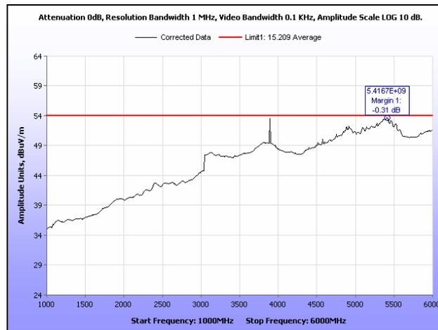
**Plot 164. Radiated Spurious Emissions, High Channel, 20 MHz, 1 GHz – 6 GHz, Average, 28 dBi**
