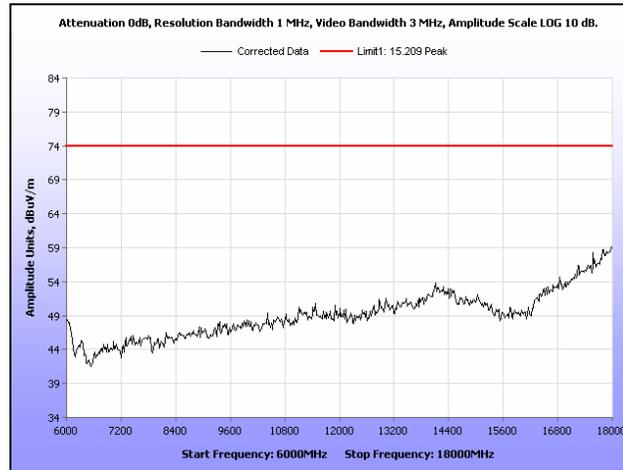
Plot 195. Radiated Spurious Emissions, Low Channel, 40 MHz, 6 GHz – 18 GHz, Peak, 21 dB
