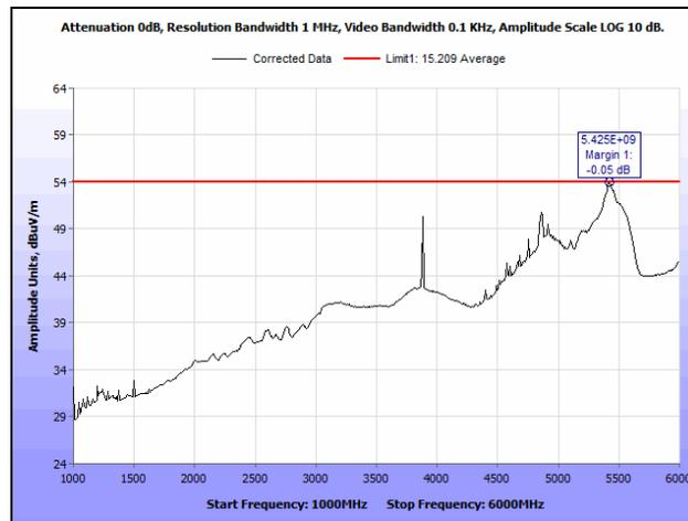
**Plot 140. Radiated Spurious Emissions, High Channel, 20 MHz, 1 GHz – 6 GHz, Average, 21 dBi**
