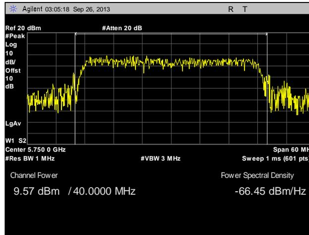
Plot 78. Peak Power Output, Point to Multi-Point, Low Channel, 40 MHz, Port 1, 21 dBi
