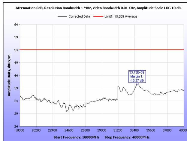
**Plot 236. Radiated Spurious Emissions, Mid Channel, 40 MHz, 18 GHz – 40 GHz, Average**
