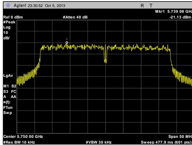
**Plot 329. Peak Power Spectral Density, Low Channel, Point to Multi-Point, 40 MHz, Port 2, 28 dBi**
