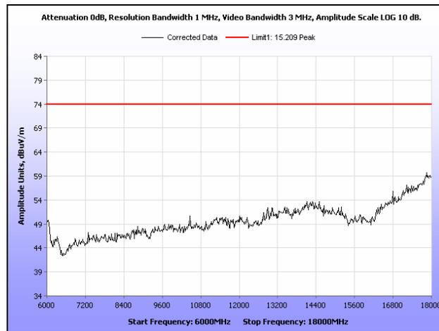
**Plot 143. Radiated Spurious Emissions, High Channel, 20 MHz, 6 GHz – 18 GHz, Peak, 21 dBi**
