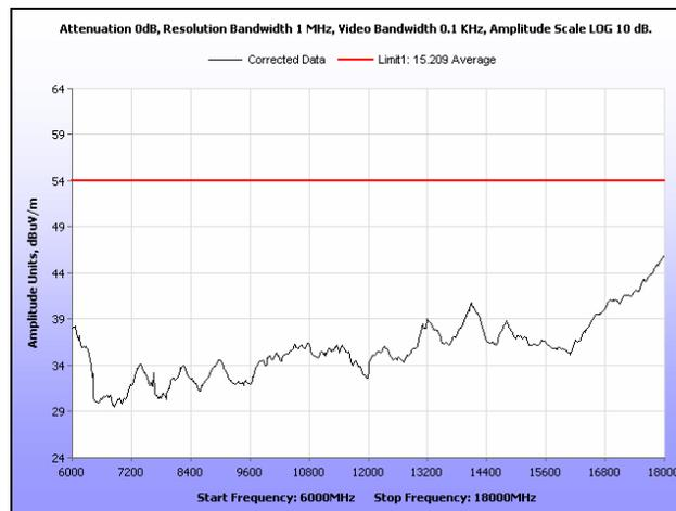
Plot 122. Radiated Spurious Emissions, Low Channel, 20 MHz, 6 GHz – 18 GHz, Average, 19 dBi
