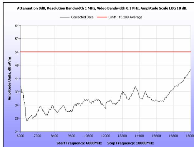
**Plot 206. Radiated Spurious Emissions, Low Channel, 40 MHz, 6 GHz – 18 GHz, Average, 23 dBi**
