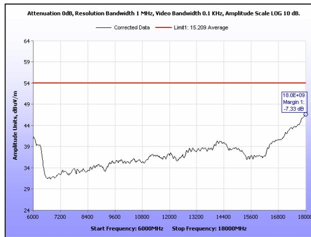
**Plot 178. Radiated Spurious Emissions, High Channel, 40 MHz, 6 GHz – 18 GHz, Average, 16 dBi**
