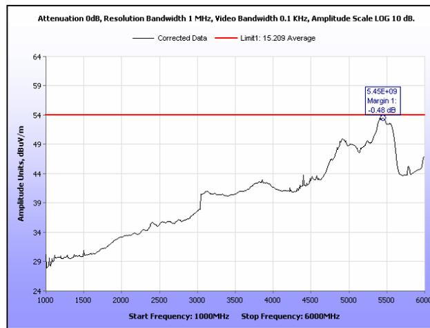
**Plot 208. Radiated Spurious Emissions, Mid Channel, 40 MHz, 1 GHz – 6 GHz, Average, 23 dB**
