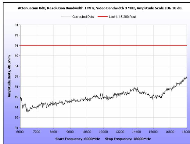
**Plot 199. Radiated Spurious Emissions, Mid Channel, 40 MHz, 6 GHz – 18 GHz, Peak, 21 dBi**
