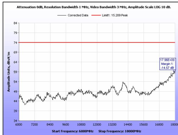
Plot 227. Radiated Spurious Emissions, High Channel, 40 MHz, 6 GHz – 18 GHz, Peak, 28 dBi
