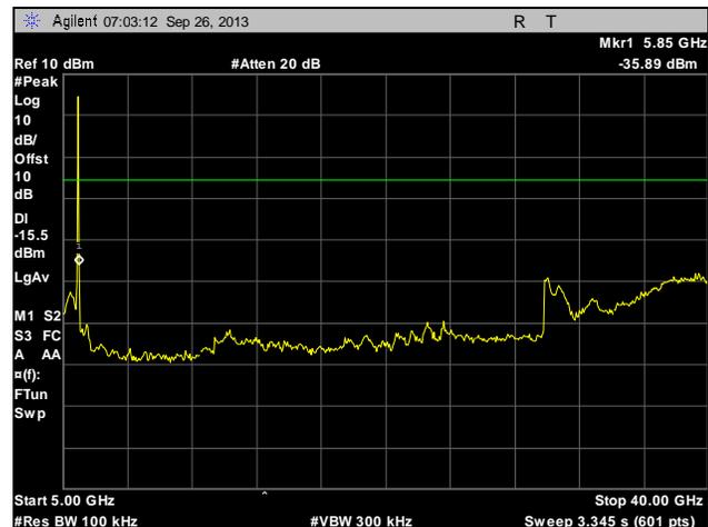
Plot 251. Conducted Spurious Emissions, High Channel, 20 MHz, Port 2, 5 GHz – 40 GHz
