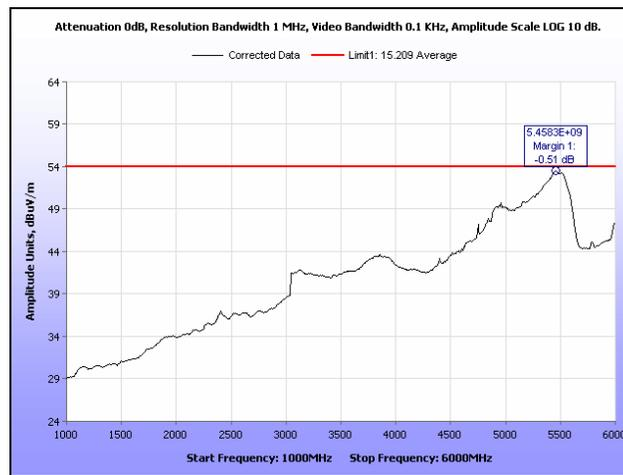
Plot 184. Radiated Spurious Emissions, Mid Channel, 40 MHz, 1 GHz – 6 GHz, Average, 19 dB
