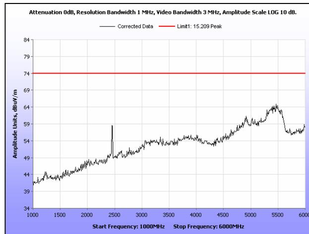
Plot 173. Radiated Spurious Emissions, Mid Channel, 40 MHz, 1 GHz – 6 GHz, Peak, 16 dB
