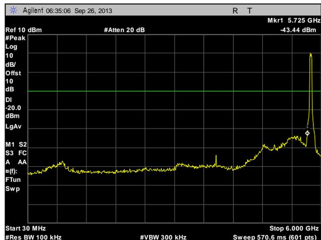
**Plot 254. Conducted Spurious Emissions, Mid Channel, 40 MHz, Port 1, 30 MHz – 6 GHz**
