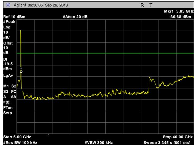
Plot 255. Conducted Spurious Emissions, Mid Channel, 40 MHz, Port 1, 5 GHz – 40 GHz
