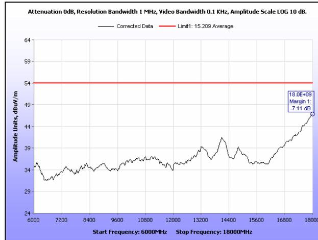
**Plot 162. Radiated Spurious Emissions, Mid Channel, 20 MHz, 6 GHz – 18 GHz, Average, 28 dBi**
