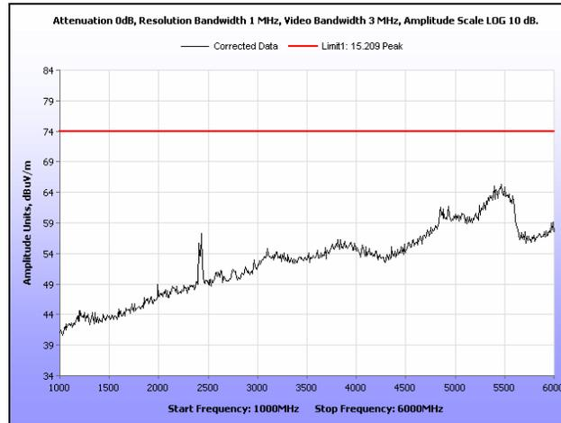
**Plot 117. Radiated Spurious Emissions, High Channel, 20 MHz, 1 GHz – 6 GHz, Peak, 16 dBi**
