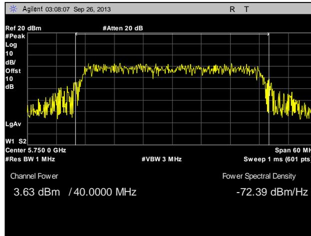
**Plot 84. Peak Power Output, Point to Multi-Point, Low Channel, 40 MHz, Port 1, 28 dBi**
