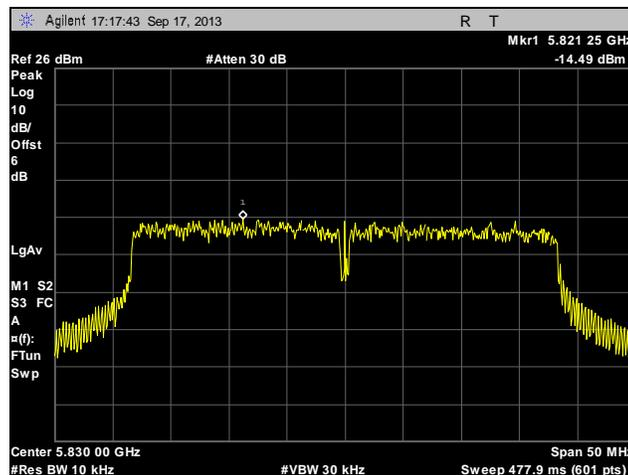
**Plot 304. Peak Power Spectral Density, High Channel, Point to Multi-Point, 40 MHz, Port 1, 16 dBi**
