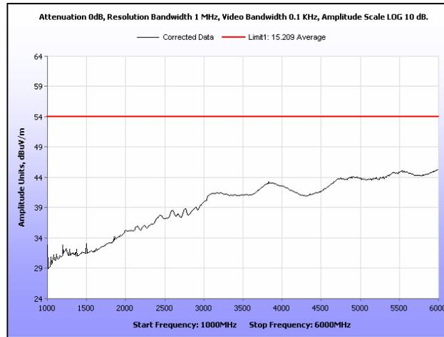
**Plot 132. Radiated Spurious Emissions, Low Channel, 20 MHz, 1 GHz – 6 GHz, Average, 21 dBi**
