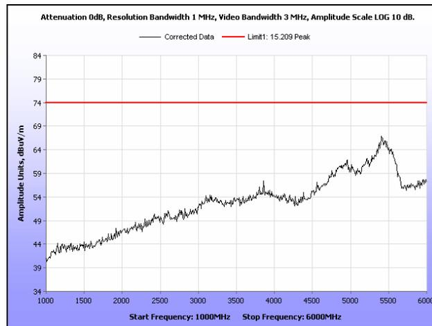
Plot 197. Radiated Spurious Emissions, Mid Channel, 40 MHz, 1 GHz – 6 GHz, Peak, 21 dB
