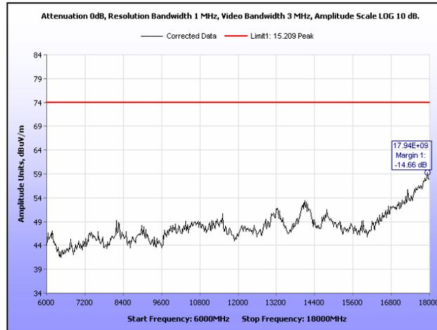
Plot 219. Radiated Spurious Emissions, Low Channel, 40 MHz, 6 GHz – 18 GHz, Peak, 28 dB
