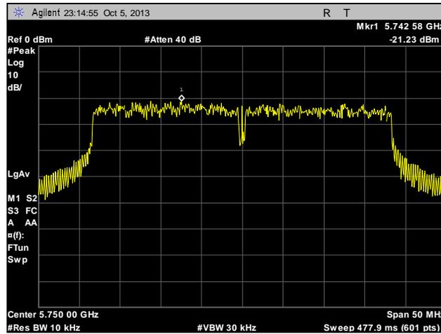
**Plot 314. Peak Power Spectral Density, Low Channel, Point to Multi-Point, 40 MHz, Port 1, 28 dBi**
