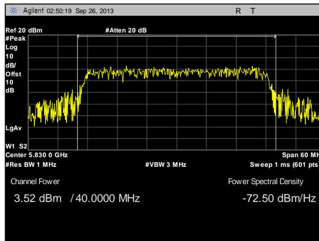
**Plot 101. Peak Power Output, Point to Multi-Point, High Channel, 40 MHz, Port 2, 28 dBi**
