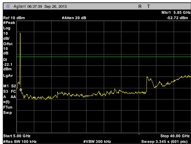
**Plot 253. Conducted Spurious Emissions, Low Channel, 40 MHz, Port 1, 5 GHz – 40 GHz**
