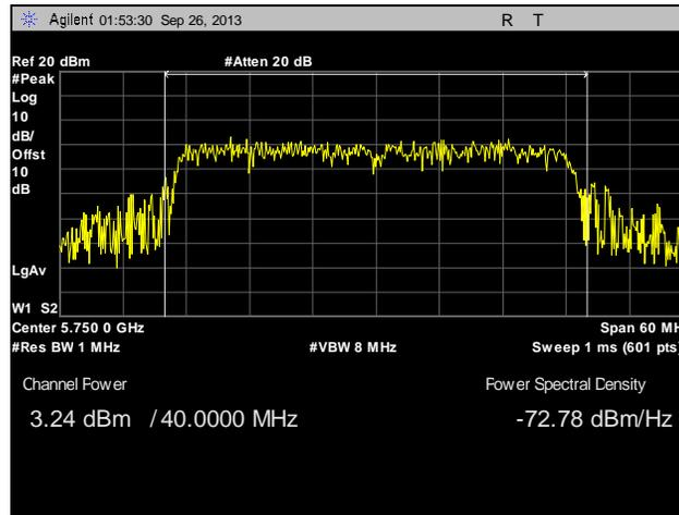
**Plot 99. Peak Power Output, Point to Multi-Point, Low Channel, 40 MHz, Port 2, 28 dBi**
