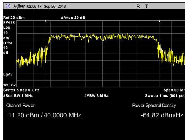
**Plot 74. Peak Power Output, Point to Multi-Point, High Channel, 40 MHz, Port 1, Port 1, 16 dBi**
