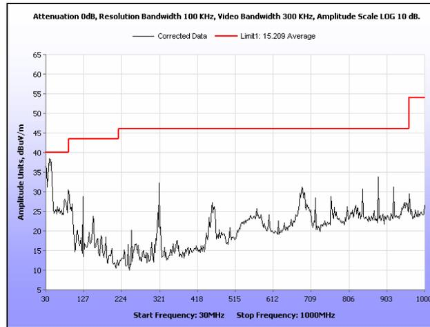
Plot 105. Radiated Spurious Emissions, Low Channel, 40 MHz, 30 MHz – 1 GHz, Peak
