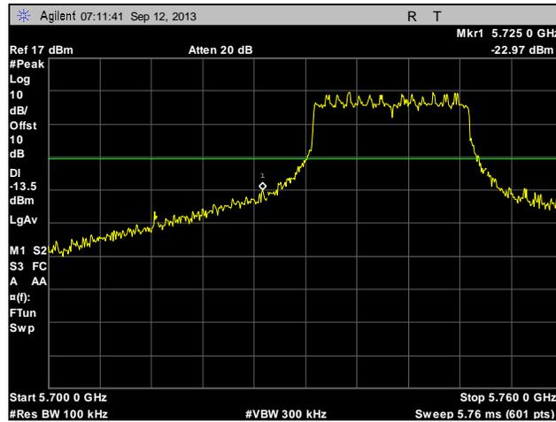
Plot 266. Conducted Band Edge, Low Channel, 20 MHz, Port 2
