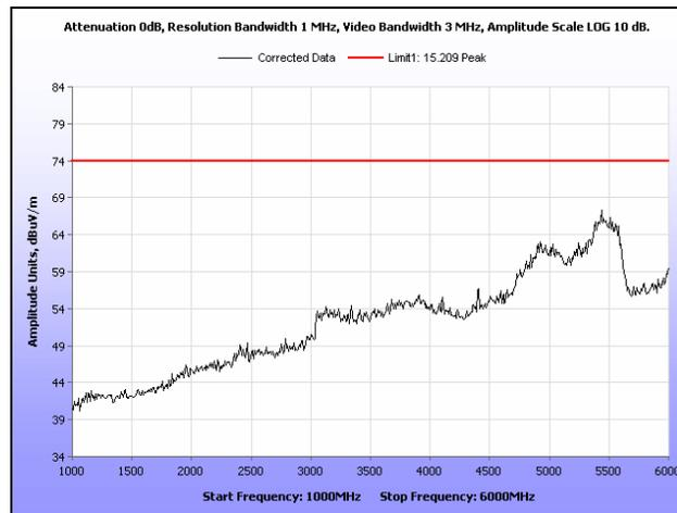
**Plot 209. Radiated Spurious Emissions, Mid Channel, 40 MHz, 1 GHz – 6 GHz, Peak, 23 dB**
