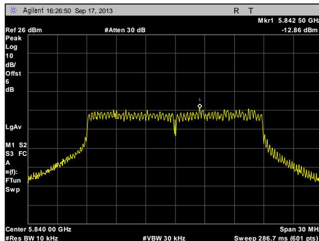
**Plot 298. Peak Power Spectral Density, High Channel, Point to Multi-Point, 20 MHz, Port 2, 23 dBi**
