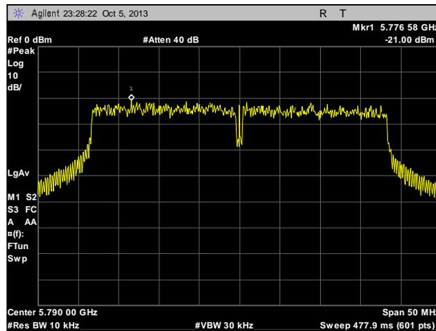
**Plot 330. Peak Power Spectral Density, Mid Channel, Point to Multi-Point, 40 MHz, Port 2, 28 dBi**
