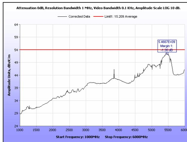
Plot 172. Radiated Spurious Emissions, Mid Channel, 40 MHz, 1 GHz – 6 GHz, Average, 16 dB
