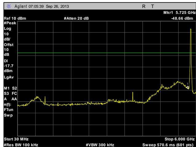
Plot 250. Conducted Spurious Emissions, High Channel, 20 MHz, Port 2, 30 MHz – 6 GHz
