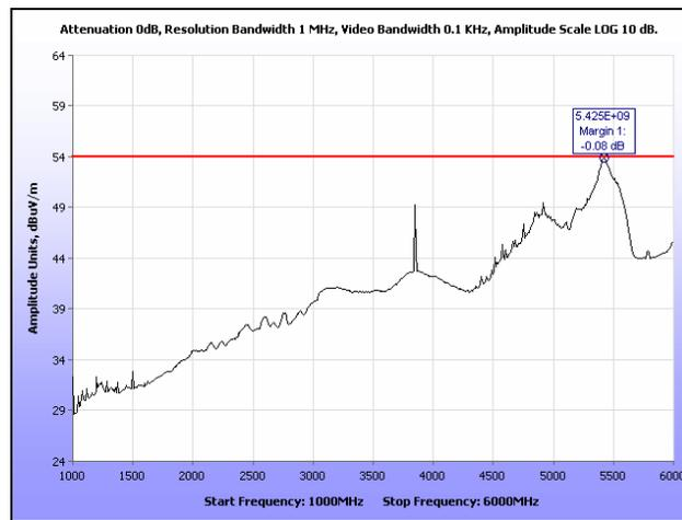
Plot 136. Radiated Spurious Emissions, Mid Channel, 20 MHz, 1 GHz – 6 GHz, Average, 21 dB
