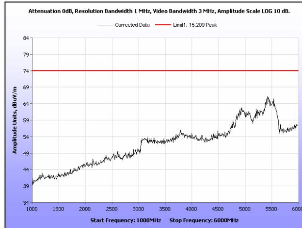
**Plot 213. Radiated Spurious Emissions, High Channel, 40 MHz, 1 GHz – 6 GHz, Peak, 23 dBi**
