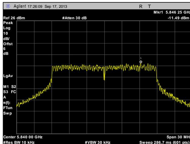
**Plot 280. Peak Power Spectral Density, High Channel, Point to Multi-Point, 20 MHz, Port 1, 21 dBi**
