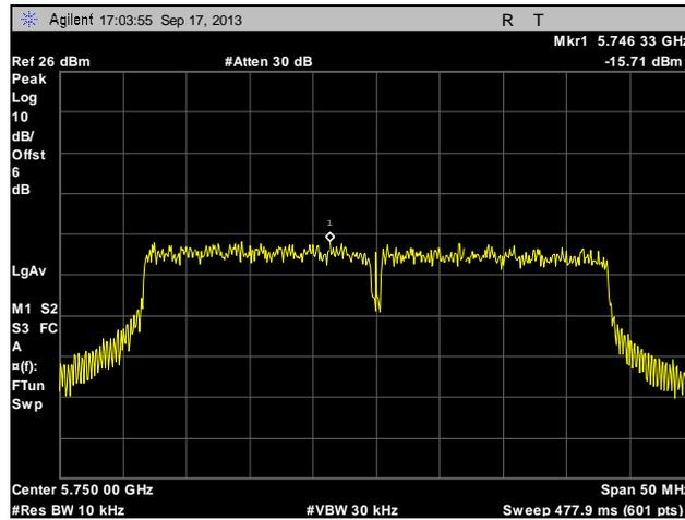
**Plot 323. Peak Power Spectral Density, Low Channel, Point to Multi-Point, 40 MHz, Port 2, 21 dBi**
