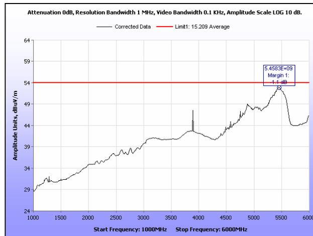
Plot 116. Radiated Spurious Emissions, High Channel, 20 MHz, 1 GHz – 6 GHz, Average, 16 dBi
