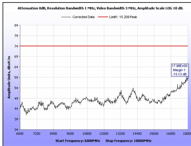
Plot 223. Radiated Spurious Emissions, Mid Channel, 40 MHz, 6 GHz – 18 GHz, Peak, 28 dBi
