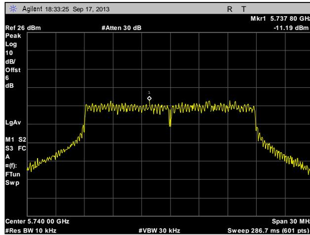
**Plot 278. Peak Power Spectral Density, Low Channel, Point to Multi-Point, 20 MHz, Port 1, 21 dBi**
