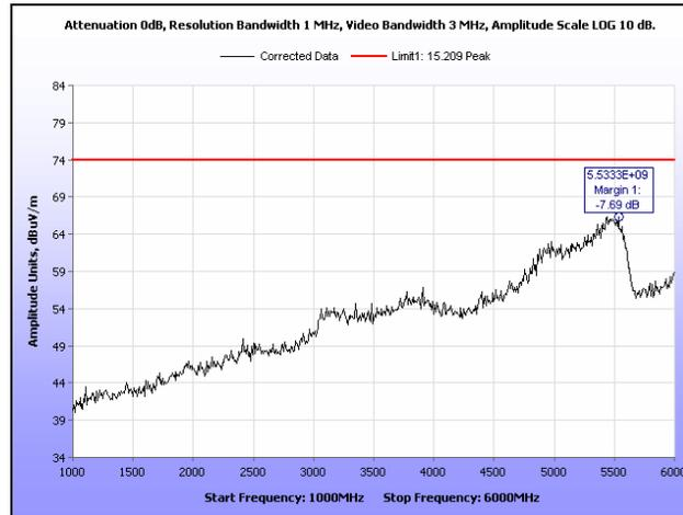
**Plot 129. Radiated Spurious Emissions, High Channel, 20 MHz, 1 GHz – 6 GHz, Peak, 19 dBi**
