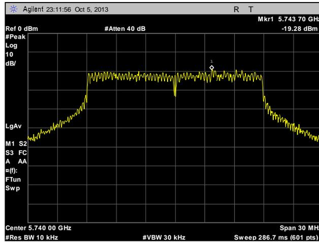
**Plot 284. Peak Power Spectral Density, Low Channel, Point to Multi-Point, 20 MHz, Port 1, 28 dBi**
