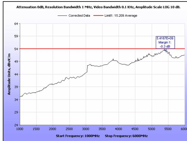
**Plot 156. Radiated Spurious Emissions, Low Channel, 20 MHz, 1 GHz – 6 GHz, Average, 28 dBi**
