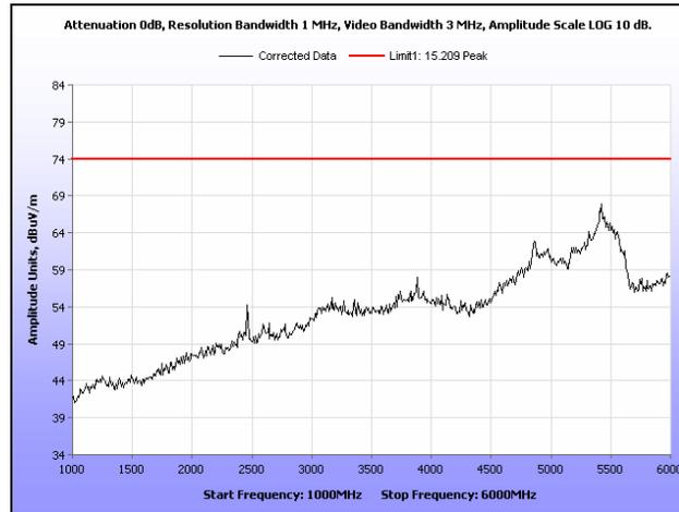
**Plot 201. Radiated Spurious Emissions, High Channel, 40 MHz, 1 GHz – 6 GHz, Peak, 21 dBi**
