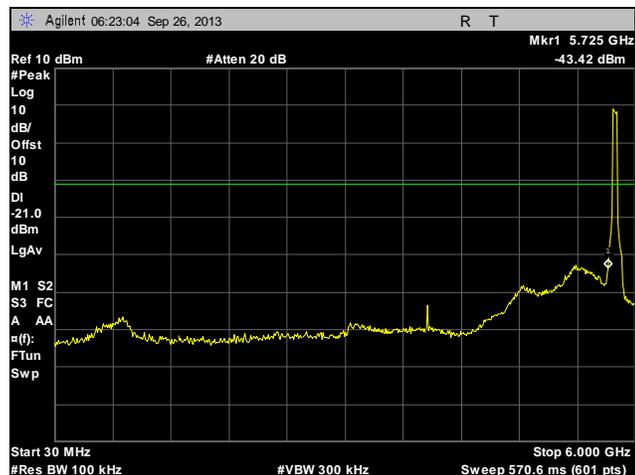
Plot 242. Conducted Spurious Emissions, Mid Channel, 20 MHz, Port 1, 30 MHz – 6 GHz
