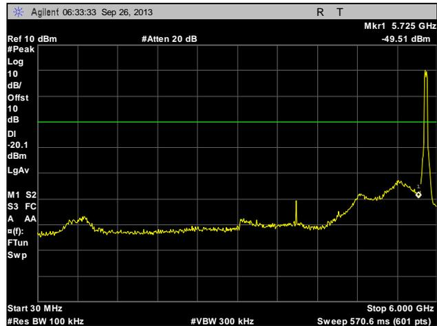
Plot 256. Conducted Spurious Emissions, High Channel, 40 MHz, Port 1, 30 MHz – 6 GHz
