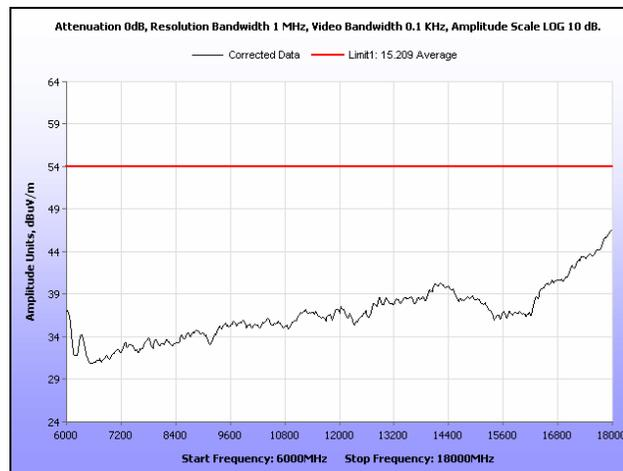
**Plot 194. Radiated Spurious Emissions, Low Channel, 40 MHz, 6 GHz – 18 GHz, Average, 21 dBi**
