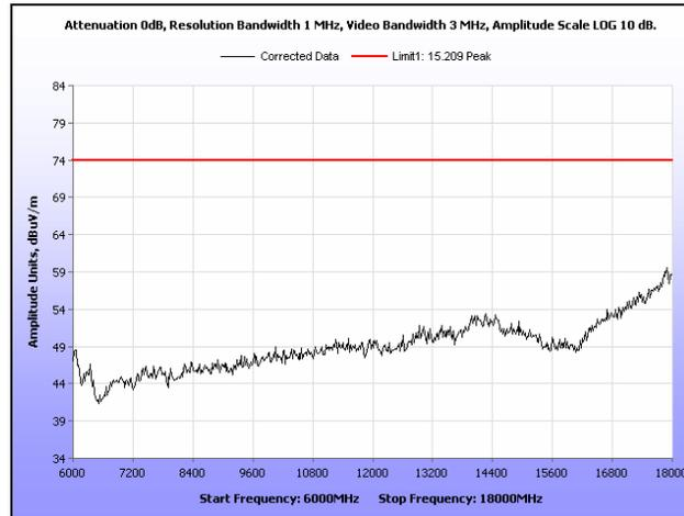
Plot 135. Radiated Spurious Emissions, Low Channel, 20 MHz, 6 GHz – 18 GHz, Peak, 21 dB
