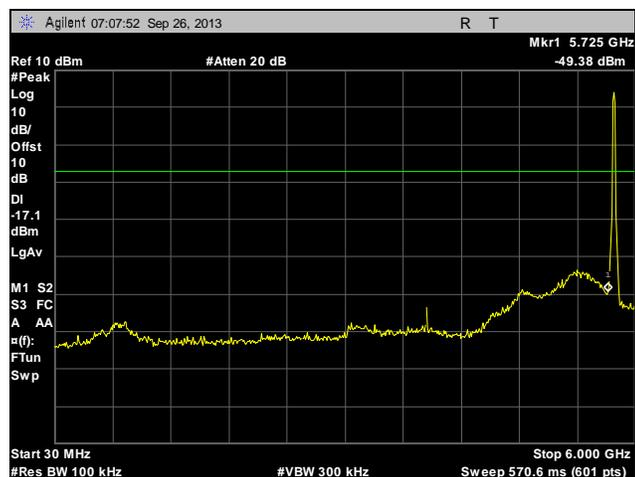
**Plot 248. Conducted Spurious Emissions, Mid Channel, 20 MHz, Port 2, 30 MHz – 6 GHz**
