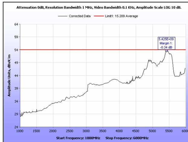
**Plot 152. Radiated Spurious Emissions, High Channel, 20 MHz, 1 GHz – 6 GHz, Average, 23 dBi**
