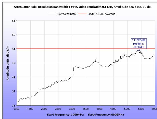
Plot 220. Radiated Spurious Emissions, Mid Channel, 40 MHz, 1 GHz – 6 GHz, Average, 28 dB
