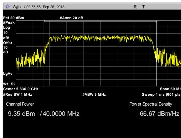
**Plot 83. Peak Power Output, Point to Multi-Point, High Channel, 40 MHz, Port 1, 23 dBi**
