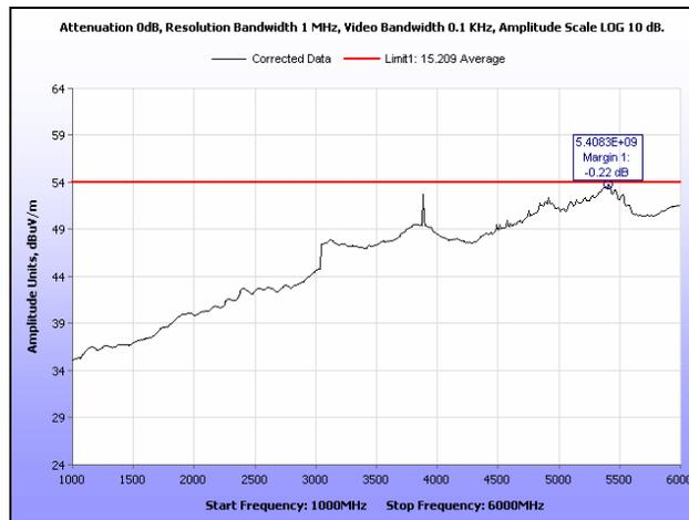
Plot 224. Radiated Spurious Emissions, High Channel, 40 MHz, 1 GHz – 6 GHz, Average, 28 dBi
