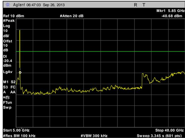
Plot 261. Conducted Spurious Emissions, Mid Channel, 40 MHz, Port 2, 5 GHz – 40 GHz
