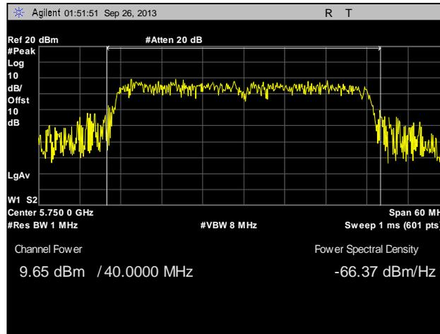
**Plot 90. Peak Power Output, Point to Multi-Point, Low Channel, 40 MHz, Port 2, 19 dBi**
