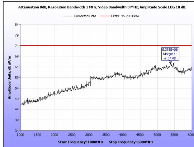
Plot 225. Radiated Spurious Emissions, High Channel, 40 MHz, 1 GHz – 6 GHz, Peak, 28 dBi
