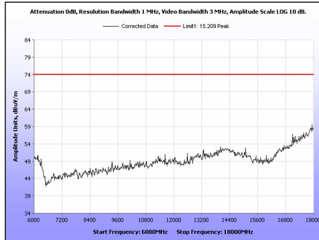
Plot 171. Radiated Spurious Emissions, Low Channel, 40 MHz, 6 GHz – 18 GHz, Peak, 16 dB
