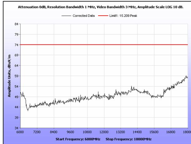
Plot 111. Radiated Spurious Emissions, Low Channel, 20 MHz, 6 GHz – 18 GHz, Peak, 16 dB
