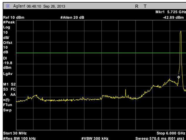
**Plot 260. Conducted Spurious Emissions, Mid Channel, 40 MHz, Port 2, 30 MHz – 6 GHz**
