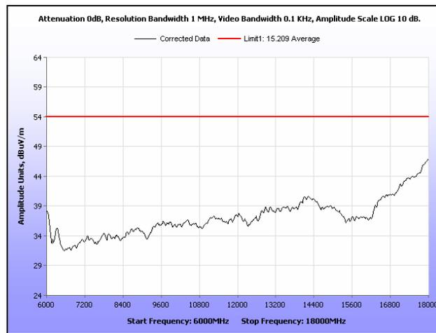
**Plot 202. Radiated Spurious Emissions, High Channel, 40 MHz, 6 GHz – 18 GHz, Average, 21 dBi**
