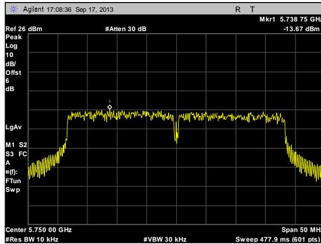
**Plot 302. Peak Power Spectral Density, Low Channel, Point to Multi-Point, 40 MHz, Port 1, 16 dBi**
