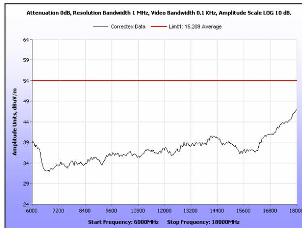
**Plot 170. Radiated Spurious Emissions, Low Channel, 40 MHz, 6 GHz – 18 GHz, Average, 16 dBi**
