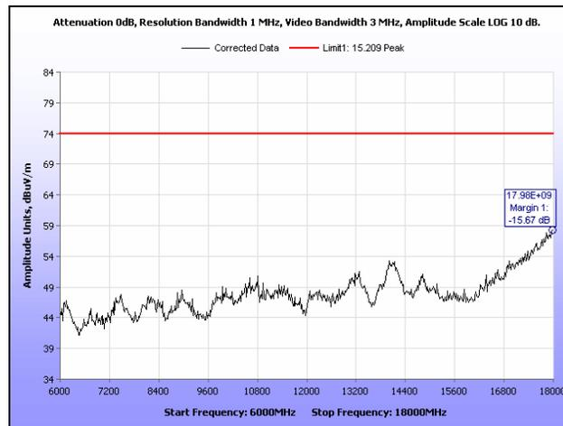
**Plot 167. Radiated Spurious Emissions, High Channel, 20 MHz, 6 GHz – 18 GHz, Peak, 28 dB**
