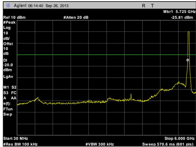
Plot 240. Conducted Spurious Emissions, Low Channel, 20 MHz, Port 1, 30 MHz – 6 GHz
