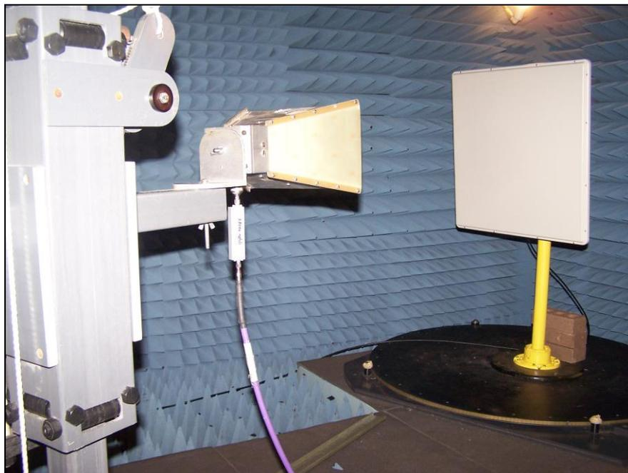
**Photograph 4. Radiated Emissions, Test Setup, 1 GHz – 2 GHz**
