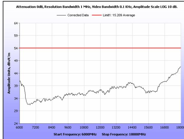
Plot 174. Radiated Spurious Emissions, Mid Channel, 40 MHz, 6 GHz – 18 GHz, Average, 16 dBi
