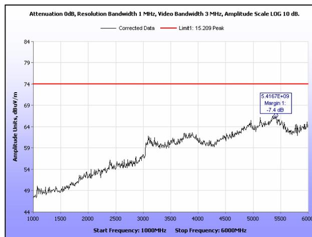
**Plot 161. Radiated Spurious Emissions, Mid Channel, 20 MHz, 1 GHz – 6 GHz, Peak, 28 dB**
