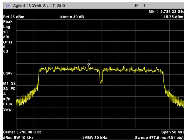
**Plot 321. Peak Power Spectral Density, Mid Channel, Point to Multi-Point, 40 MHz, Port 2, 19 dBi**
