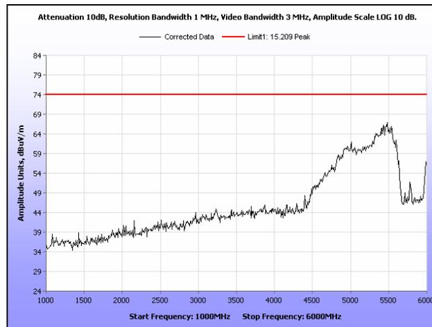
Plot 185. Radiated Spurious Emissions, Mid Channel, 40 MHz, 1 GHz – 6 GHz, Peak, 19 dB
