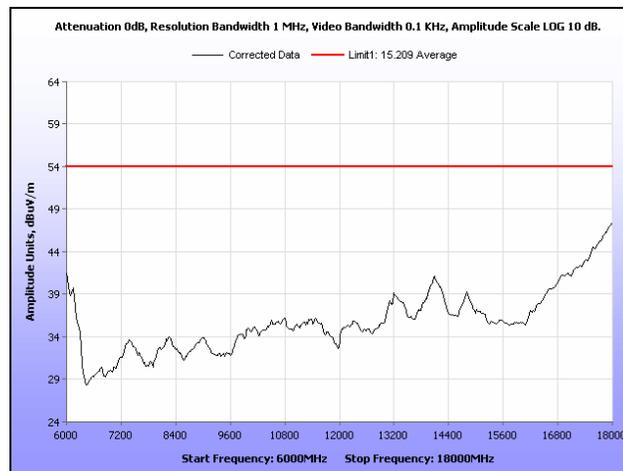
**Plot 146. Radiated Spurious Emissions, Low Channel, 20 MHz, 6 GHz – 18 GHz, Average, 23 dBi**
