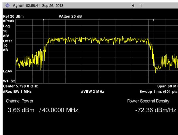
**Plot 85. Peak Power Output, Point to Multi-Point, Mid Channel, 40 MHz, Port 1, 28 dBi**
