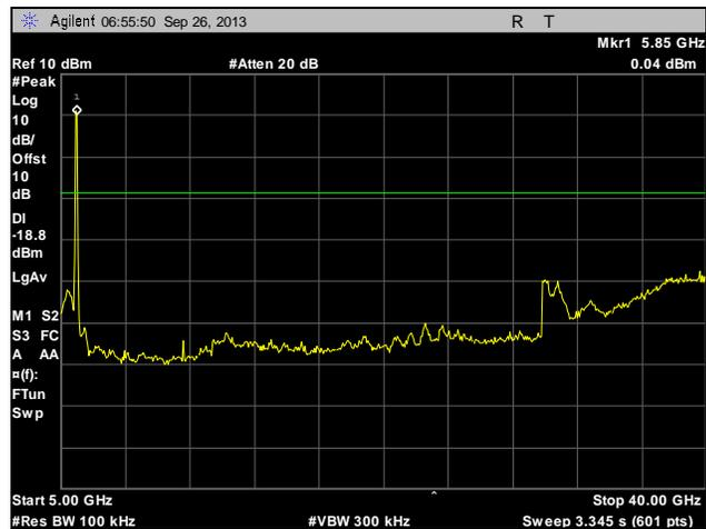
Plot 263. Conducted Spurious Emissions, High Channel, 40 MHz, Port 2, 5 GHz – 40 GHz
