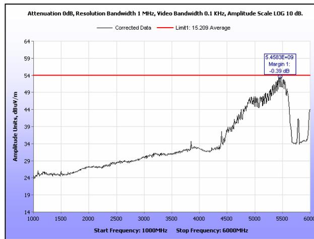
Plot 124. Radiated Spurious Emissions, Mid Channel, 20 MHz, 1 GHz – 6 GHz, Average, 19 dB
