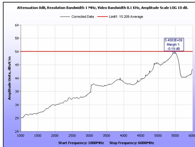
Plot 128. Radiated Spurious Emissions, High Channel, 20 MHz, 1 GHz – 6 GHz, Average, 19 dBi
