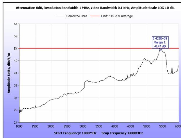
Plot 148. Radiated Spurious Emissions, Mid Channel, 20 MHz, 1 GHz – 6 GHz, Average, 23 dB
