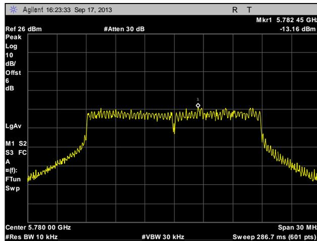
**Plot 294. Peak Power Spectral Density, Mid Channel, Point to Multi-Point, 20 MHz, Port 2, 21 dBi**
