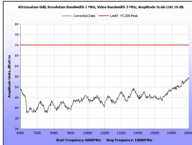
Plot 183. Radiated Spurious Emissions, Low Channel, 40 MHz, 6 GHz – 18 GHz, Peak, 19 dB
