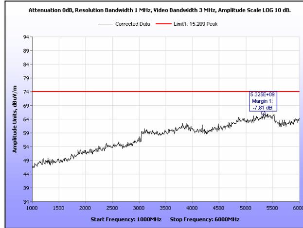
**Plot 165. Radiated Spurious Emissions, High Channel, 20 MHz, 1 GHz – 6 GHz, Peak, 28 dB**
