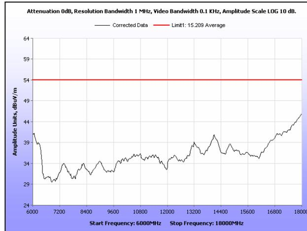
Plot 126. Radiated Spurious Emissions, Mid Channel, 20 MHz, 6 GHz – 18 GHz, Average, 19 dBi
