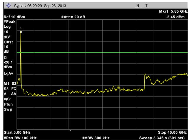
Plot 245. Conducted Spurious Emissions, High Channel, 20 MHz, Port 1, 5 GHz – 40 GHz
