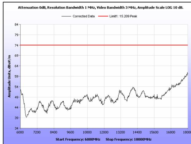
**Plot 155. Radiated Spurious Emissions, High Channel, 20 MHz, 6 GHz – 18 GHz, Peak, 23 dBi**
