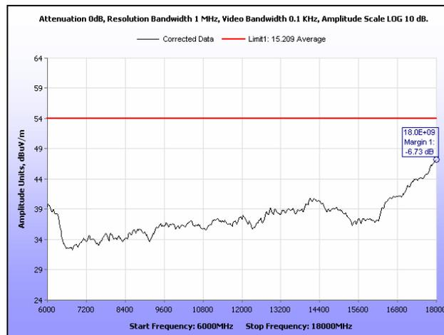
Plot 110. Radiated Spurious Emissions, Low Channel, 20 MHz, 6 GHz – 18 GHz, Average, 16 dBi
