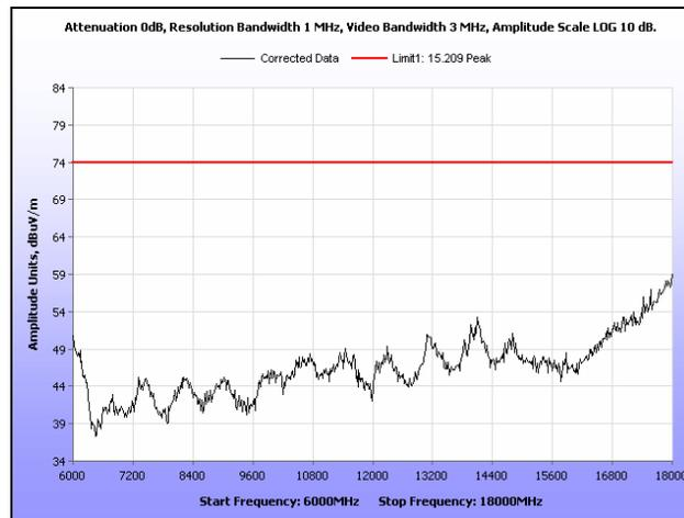
**Plot 215. Radiated Spurious Emissions, High Channel, 40 MHz, 6 GHz – 18 GHz, Peak, 23 dBi**
