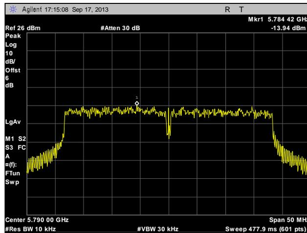
**Plot 306. Peak Power Spectral Density, Mid Channel, Point to Multi-Point, 40 MHz, Port 1, 19 dBi**
