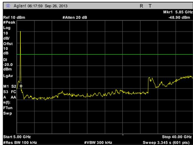
Plot 241. Conducted Spurious Emissions, Low Channel, 20 MHz, Port 1, 5 GHz – 40 GHz
