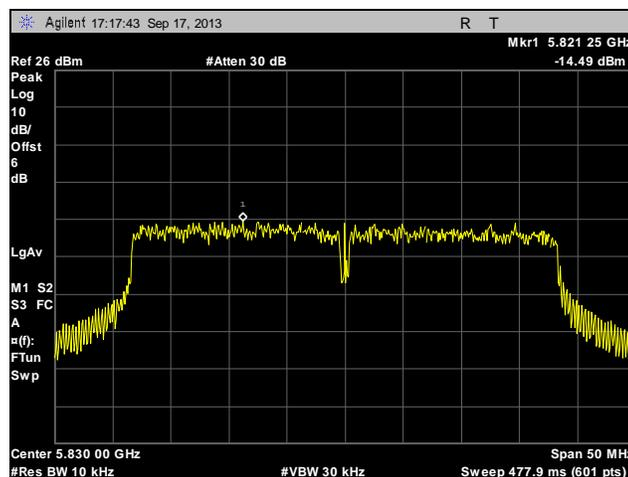
**Plot 313. Peak Power Spectral Density, High Channel, Point to Multi-Point, 40 MHz, Port 1, 23 dBi**
