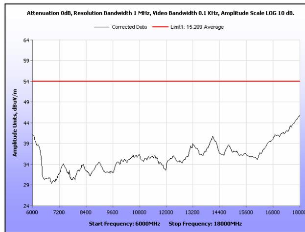
**Plot 130. Radiated Spurious Emissions, High Channel, 20 MHz, 6 GHz – 18 GHz, Average, 19 dBi**
