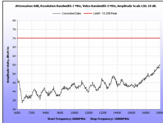
**Plot 207. Radiated Spurious Emissions, Low Channel, 40 MHz, 6 GHz – 18 GHz, Peak, 23 dB**
