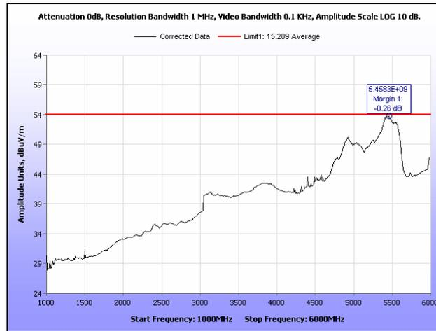
**Plot 144. Radiated Spurious Emissions, Low Channel, 20 MHz, 1 GHz – 6 GHz, Average, 23 dBi**
