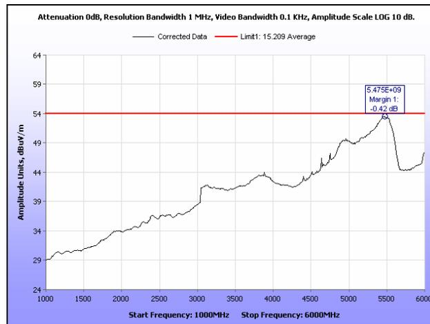
Plot 188. Radiated Spurious Emissions, High Channel, 40 MHz, 1 GHz – 6 GHz, Average, 19 dBi
