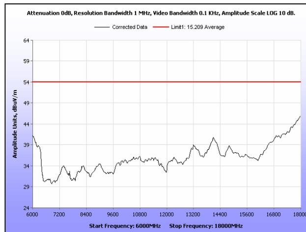
Plot 182. Radiated Spurious Emissions, Low Channel, 40 MHz, 6 GHz – 18 GHz, Average, 19 dBi
