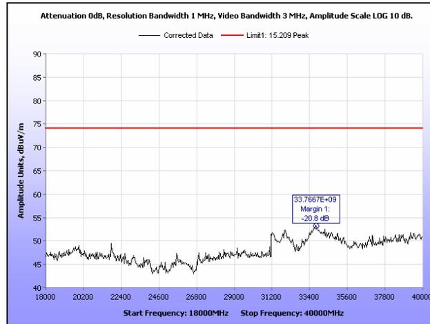
**Plot 237. Radiated Spurious Emissions, Mid Channel, 40 MHz, 18 GHz – 40 GHz, Peak**
