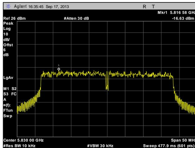
**Plot 328. Peak Power Spectral Density, High Channel, Point to Multi-Point, 40 MHz, Port 2, 23 dBi**
