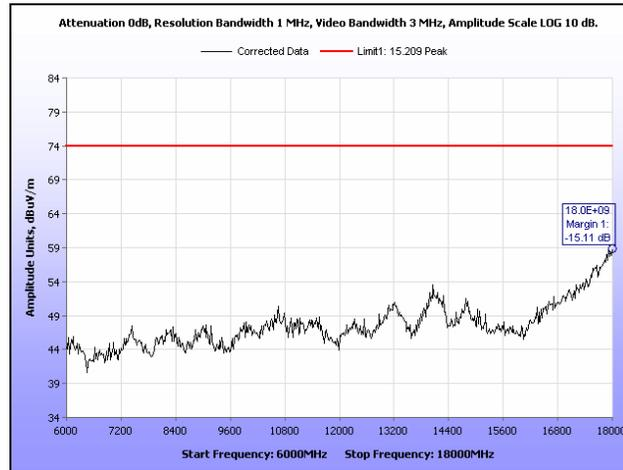
**Plot 159. Radiated Spurious Emissions, Low Channel, 20 MHz, 6 GHz – 18 GHz, Peak, 28 dB**
