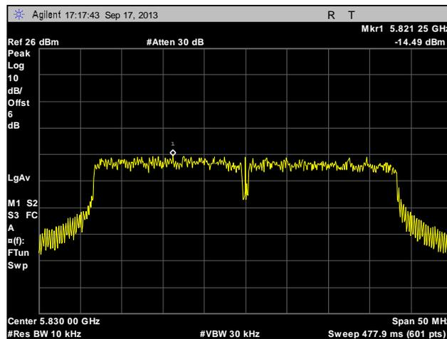
**Plot 310. Peak Power Spectral Density, High Channel, Point to Multi-Point, 40 MHz, Port 1, 21 dBi**
