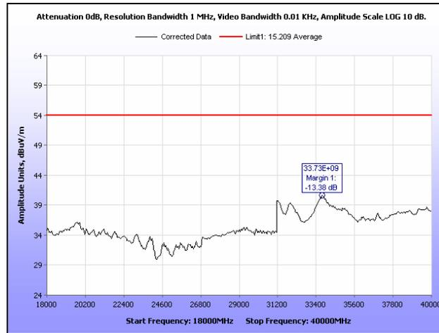
**Plot 228. Radiated Spurious Emissions, Low Channel, 20 MHz, 18 GHz – 40 GHz, Average**
