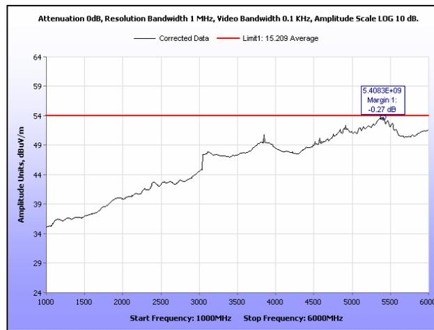
**Plot 160. Radiated Spurious Emissions, Mid Channel, 20 MHz, 1 GHz – 6 GHz, Average, 28 dB**
