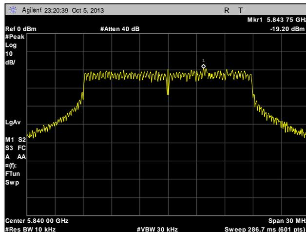
**Plot 316. Peak Power Spectral Density, High Channel, Point to Multi-Point, 40 MHz, Port 1, 28 dBi**
