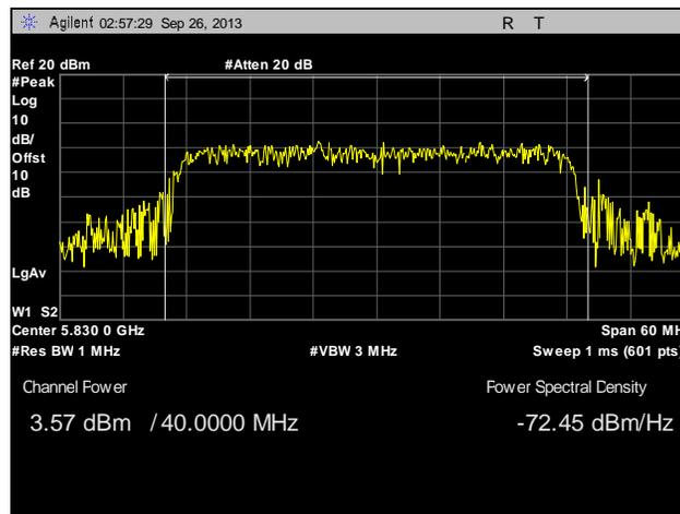
**Plot 86. Peak Power Output, Point to Multi-Point, High Channel, 40 MHz, Port 1, 28 dBi**
