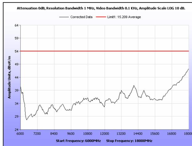
**Plot 154. Radiated Spurious Emissions, High Channel, 20 MHz, 6 GHz – 18 GHz, Average, 23 dBi**
