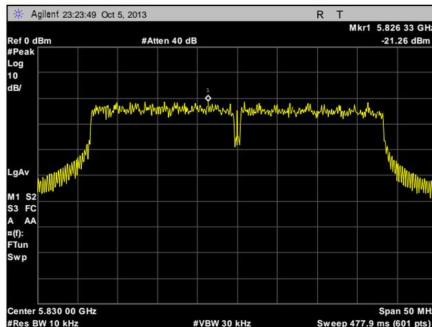
**Plot 331. Peak Power Spectral Density, High Channel, Point to Multi-Point, 40 MHz, Port 2, 28 dBi**
