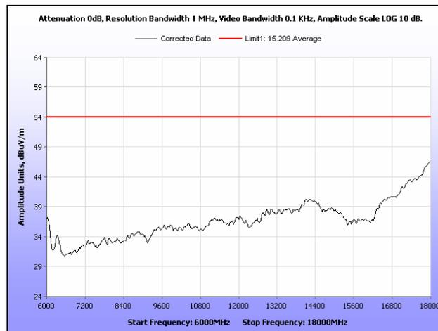
**Plot 134. Radiated Spurious Emissions, Low Channel, 20 MHz, 6 GHz – 18 GHz, Average, 21 dBi**
