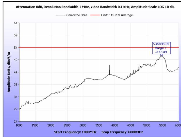
Plot 108. Radiated Spurious Emissions, Low Channel, 20 MHz, 1 GHz – 6 GHz, Average, 16 dBi
